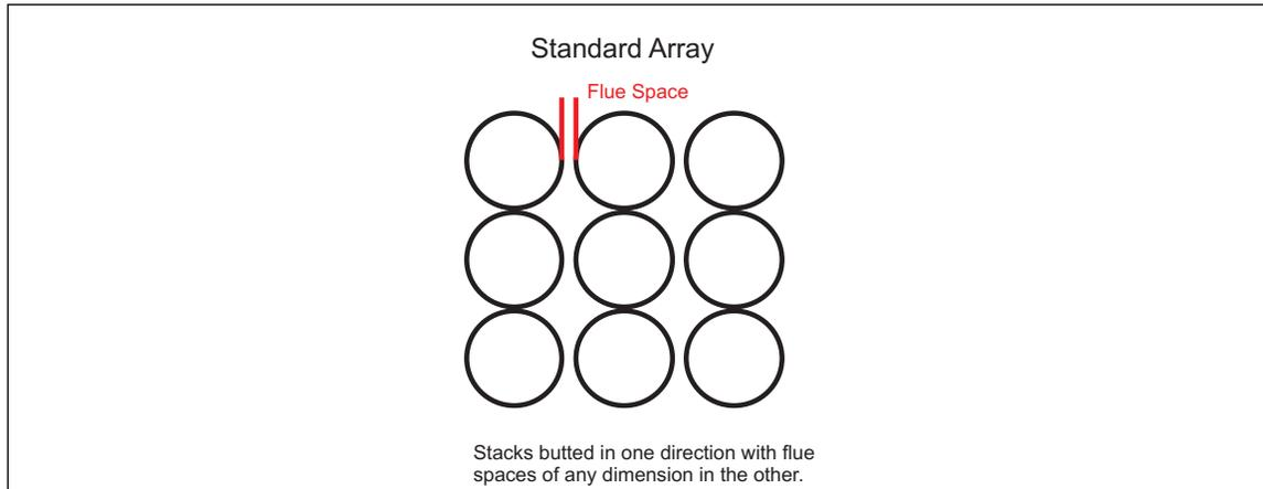
Fig. A-4. Roll paper standard array
