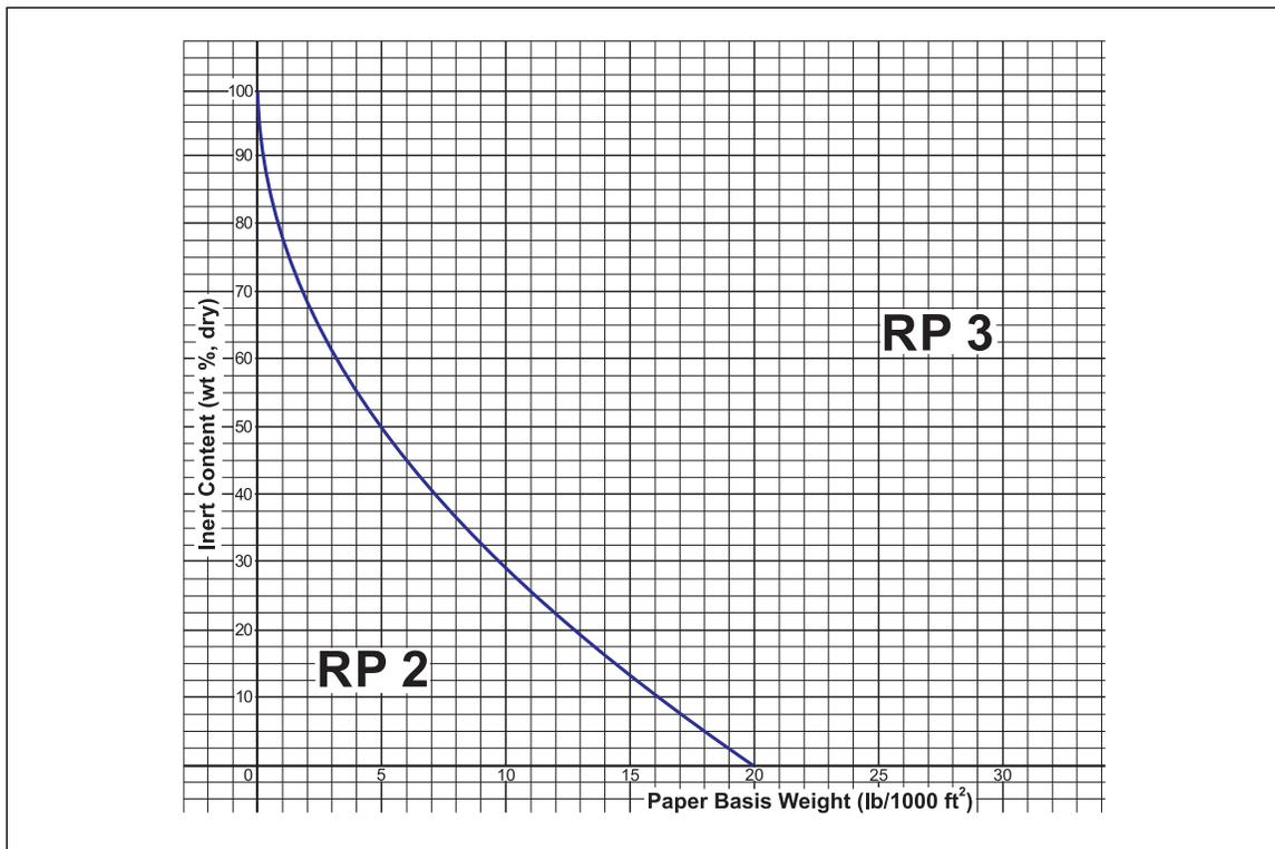
Fig. 2.2.1.2.1-1. Hard-surface roll paper classification (imperial)
