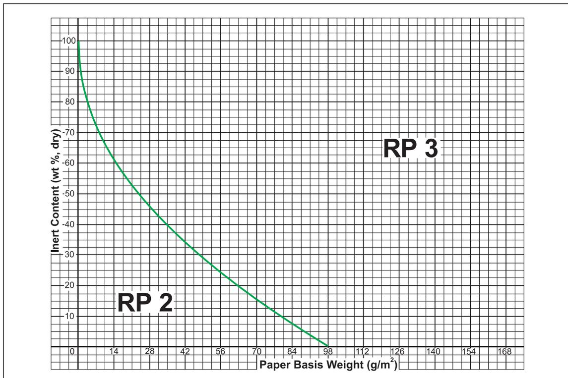
Fig. 2.2.1.2-2. Hard-surface roll paper classification (metric)
