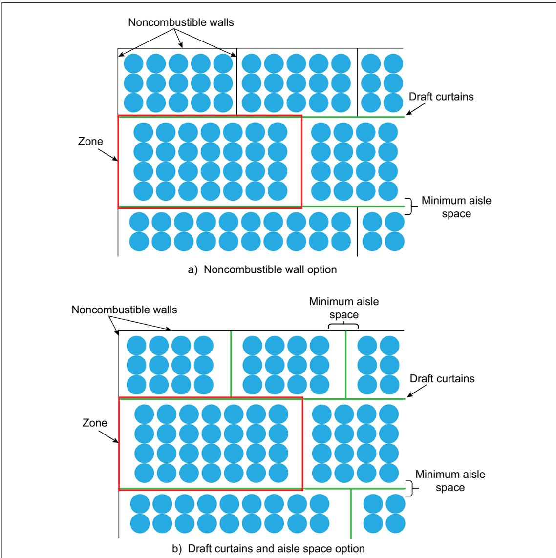
Fig. 2.2.6.1.2. Schematic of storage area separated into zones for RP 1, a) using noncombustible walls and b) using draft curtains and aisle spaces
