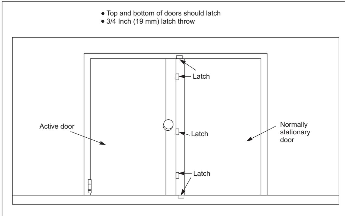
Fig. 2.1.5.1-3. Details for double doors in pressure-resistant walls
