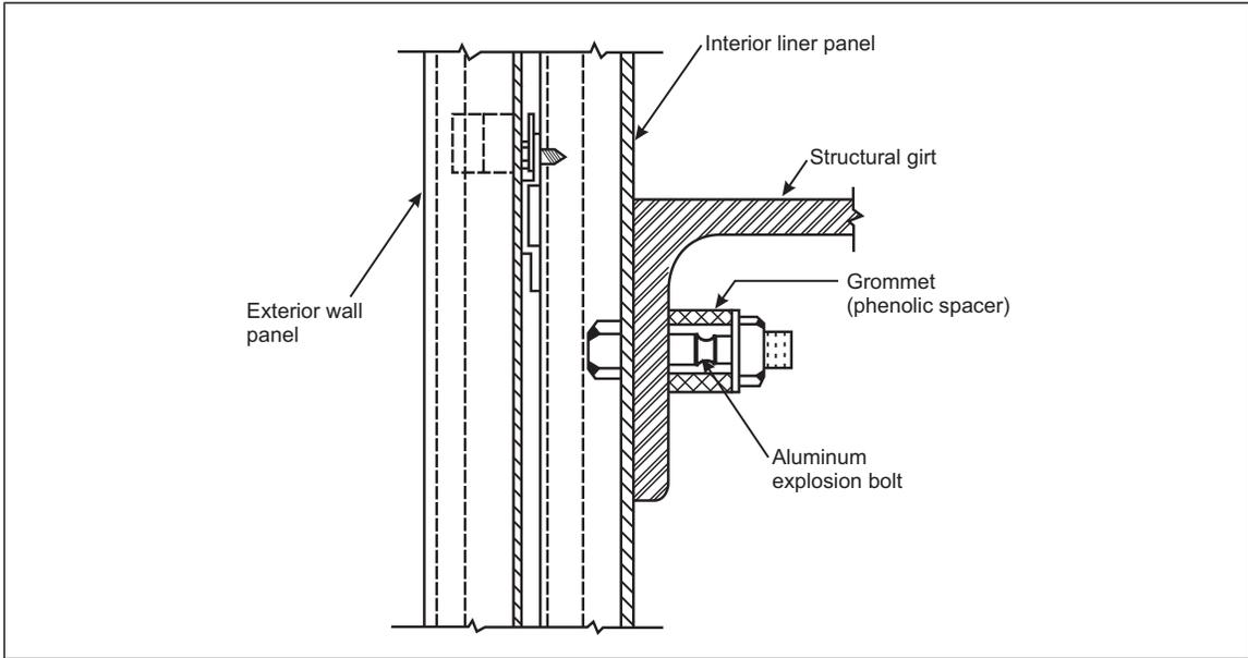
Fig. 2.1.4.1-2. Reduced-shank machine bolt installed to fail in tension
