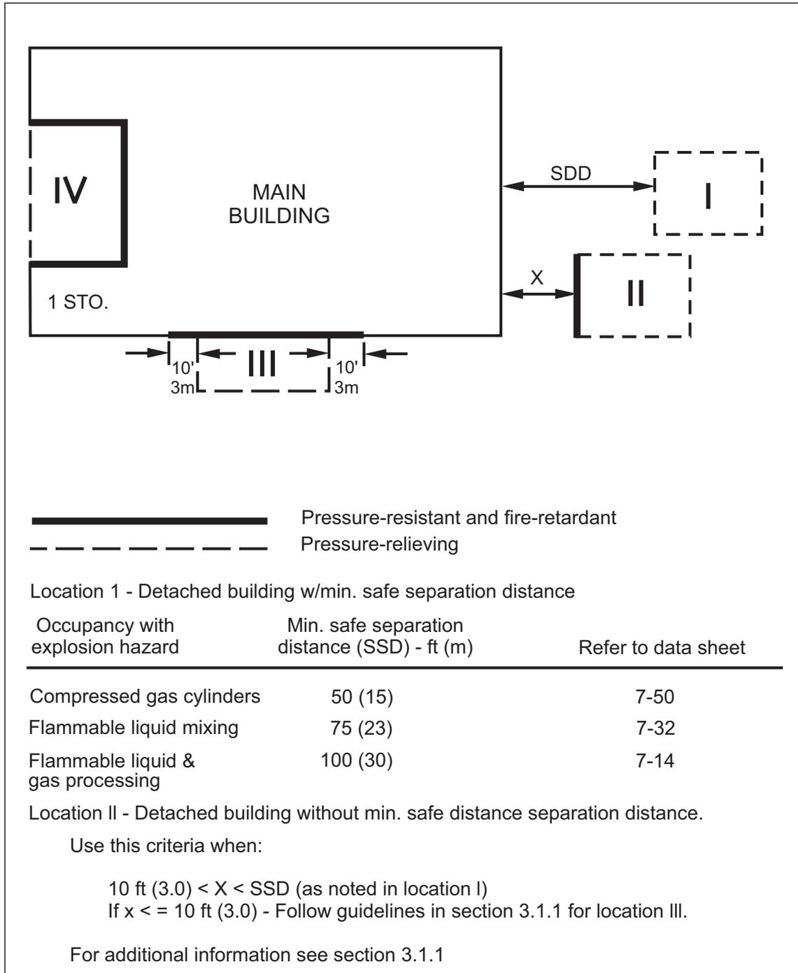
Fig. 3.1.1. Locations for damage-limiting construction, in order of preference
