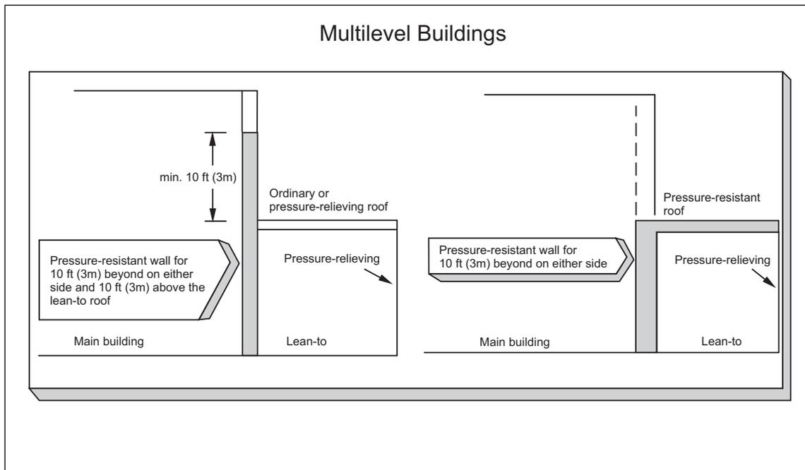
Fig. 2.1.5.1-1. Construction details for lean-to with damage-limiting construction
