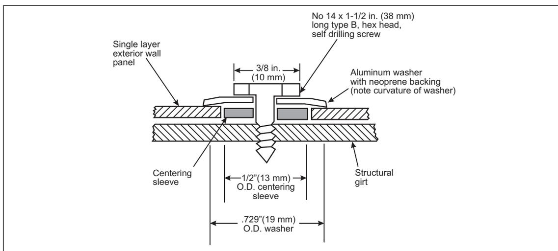
Fig. 2.1.4.1-1. Collapsing washer used with a single-layer panel
