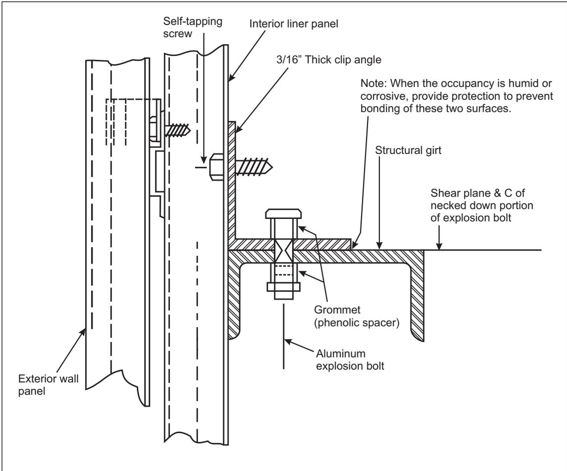
Fig. 2.1.4.1-3. Reduced-shank machine bolt installed to fail in shear.
