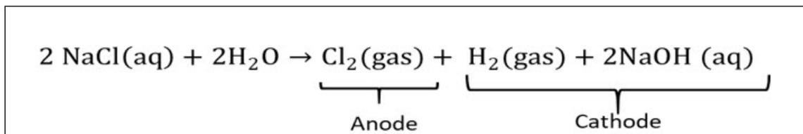
Large electrical demand is needed for the endothermic process. The AC electrical power is converted to direct current (DC) power in large rectifying transformers. Brine is electrolyzed to chlorine at the anode and to hydrogen and caustic soda at the cathode.
