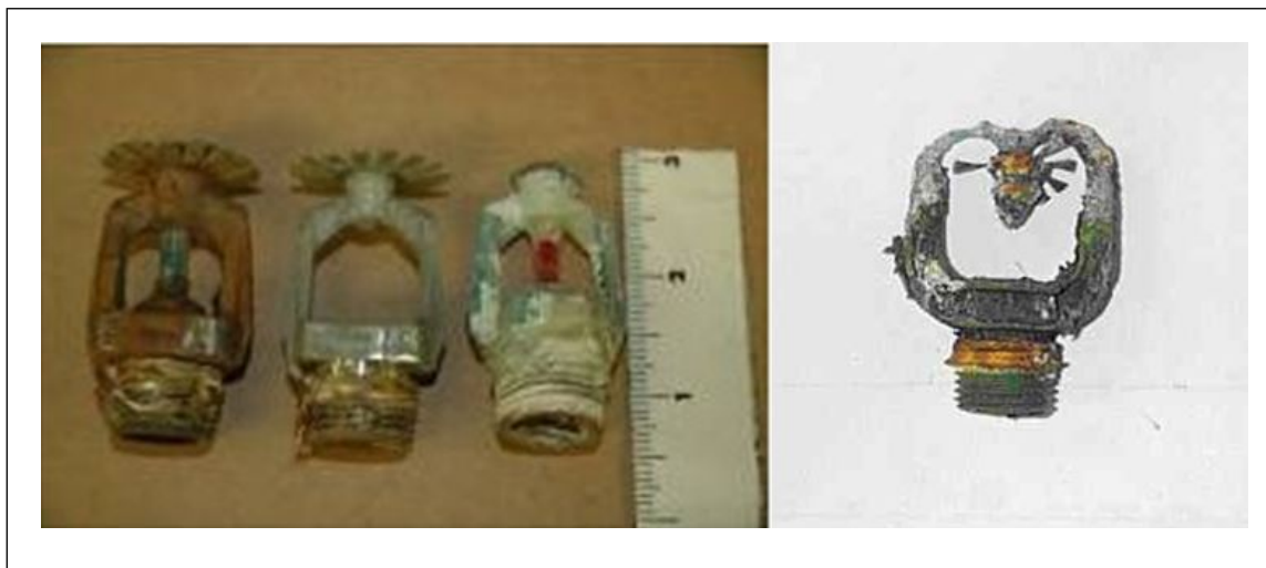
Fig. 1. Corrosion-damaged fire protection components
