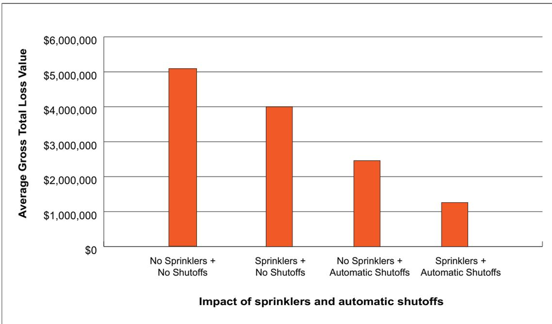
Fig. 3.3-2. Impact of shutoffs and sprinklers
