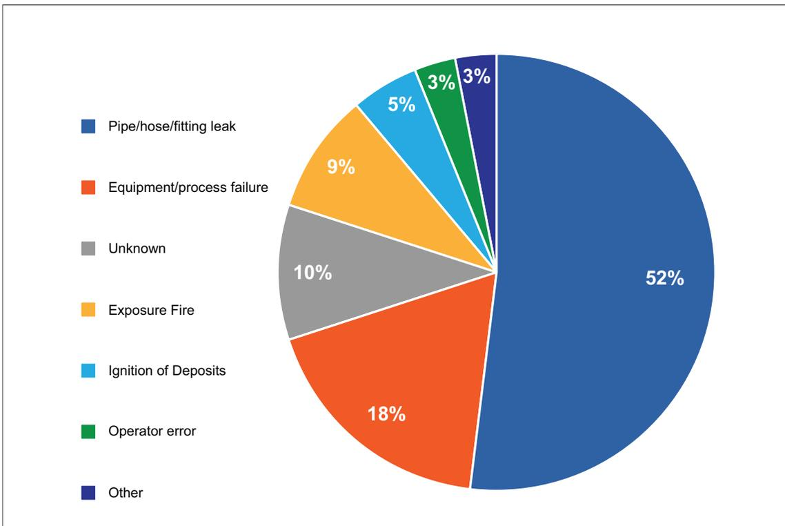
Fig. 3.3-3. Causes of hydraulic fire losses (by frequency)
