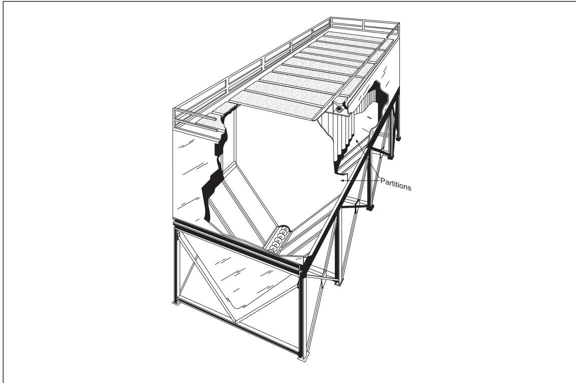
Fig. 2.2.2.3-1. Large collector showing partitions subdividing the unit
