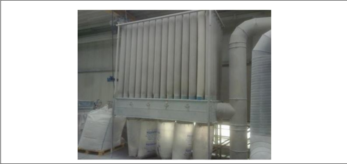
Fig. 3.4.1.1-1. Example of an enclosureless collector
