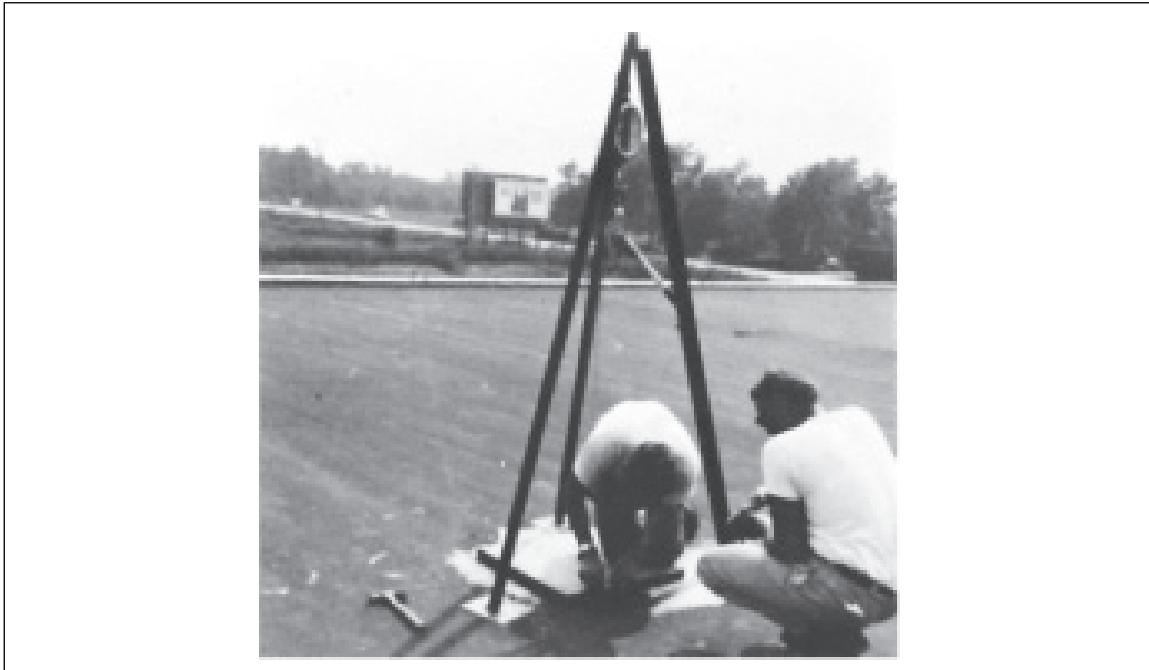
Fig. E.2.1.2-2. Bonded uplift test
