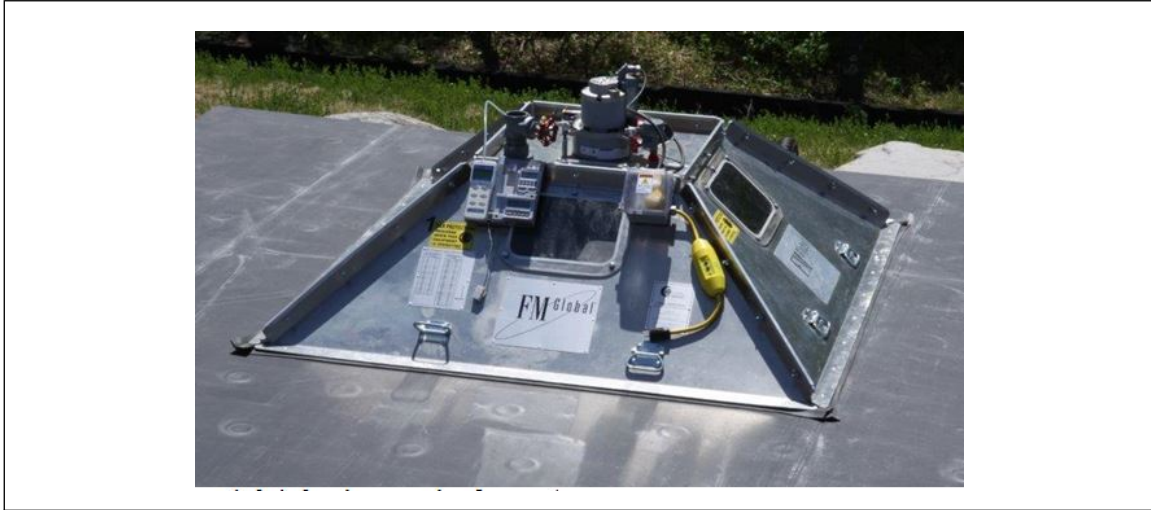
Fig. D.1.2.1-2. Photograph of negative pressure test apparatus
