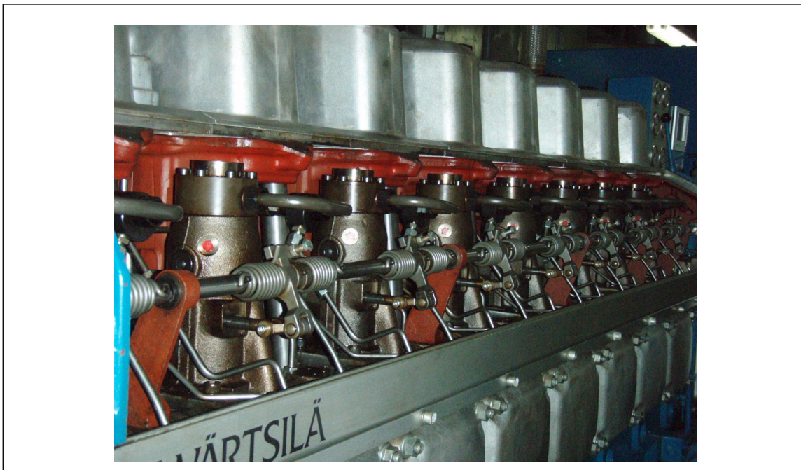
Fig. 7. Mechanical fuel injection system (courtesy Wartsila Corp.)
