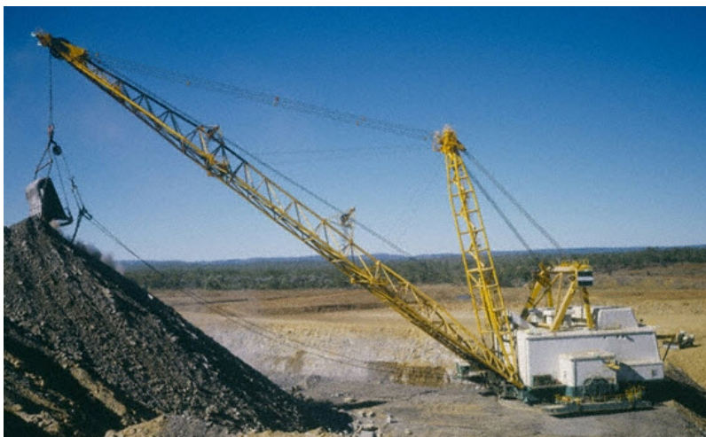
Fig. C.1-1. Walking drag line in a strip mine
