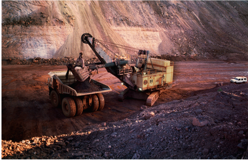
Fig. 3.1-2 Large excavating shovel loading a haul truck in a hard rock open pit mine
