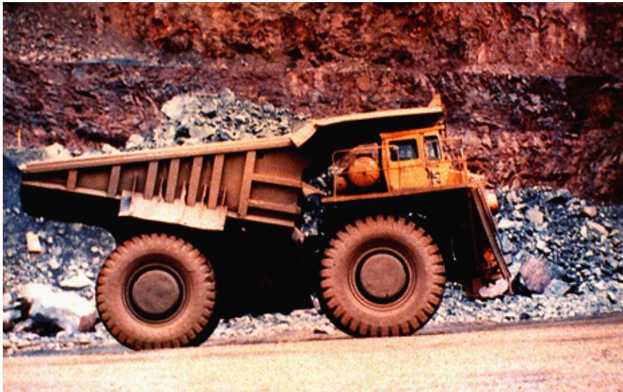
Fig. 3.1-1. Self-propelled 190 ton (172 metric tonne) ore haul truck
