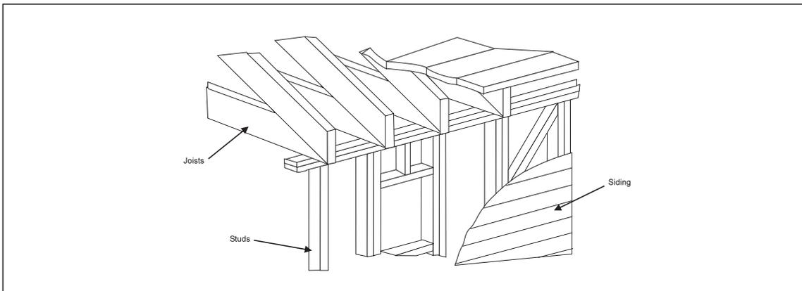
Fig. 14. Wood frame construction.
