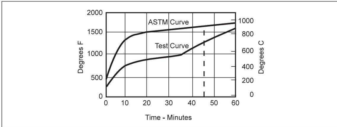
Fig. 2. The area, in degree-hours, under the test curve for 60 minutes is the same as the area under the ASTM curve for 45 minutes. Therefore, the severity of the fire exposure under both curves, up to these respective time limits, is approximately the same.
