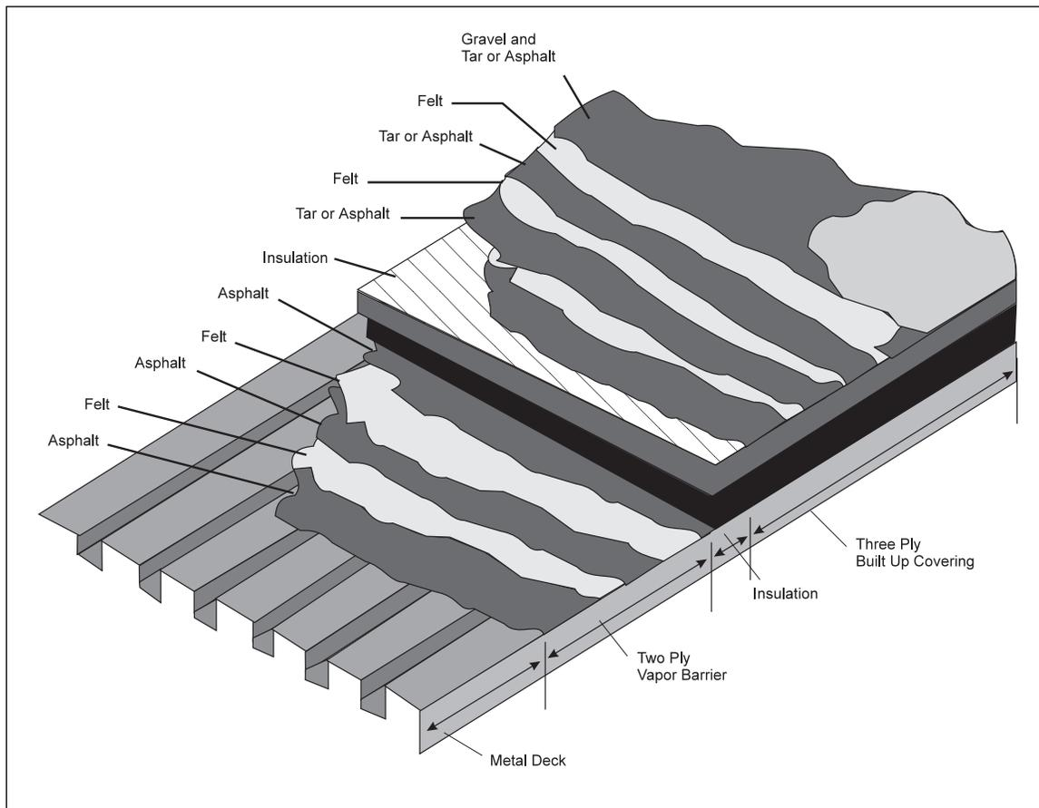
Fig. 16. Typical Class 2 insulated metal roof deck construction with vapor barrier.
