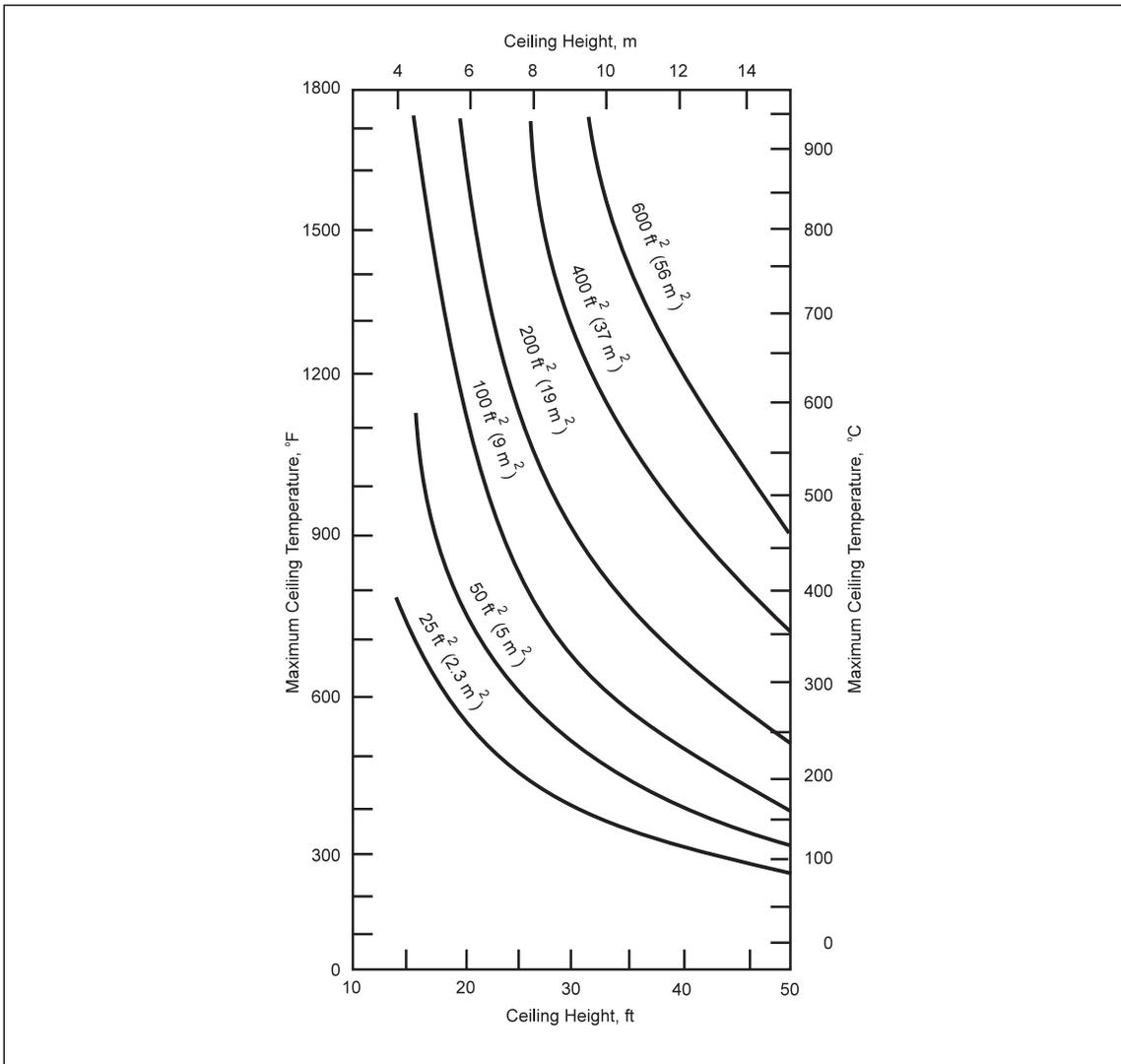
Fig. 5. Ceiling temperatures, ignitable liquid pool fires.
