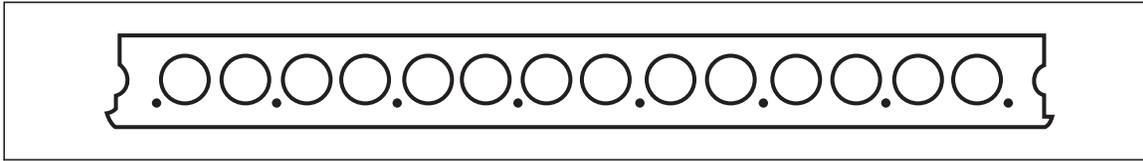
Fig. 8c. Hollow Core Flat Slab.
