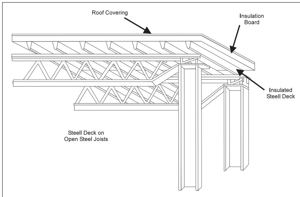
Fig. 11. Insulated steel deck on steel framing.
