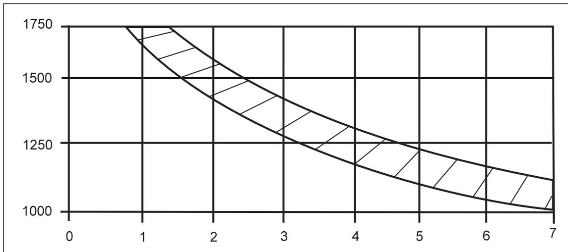
Fig. 10. Exposure required to distort structural steel to the point where breakage of sprinkler pipe fittings will occur.
