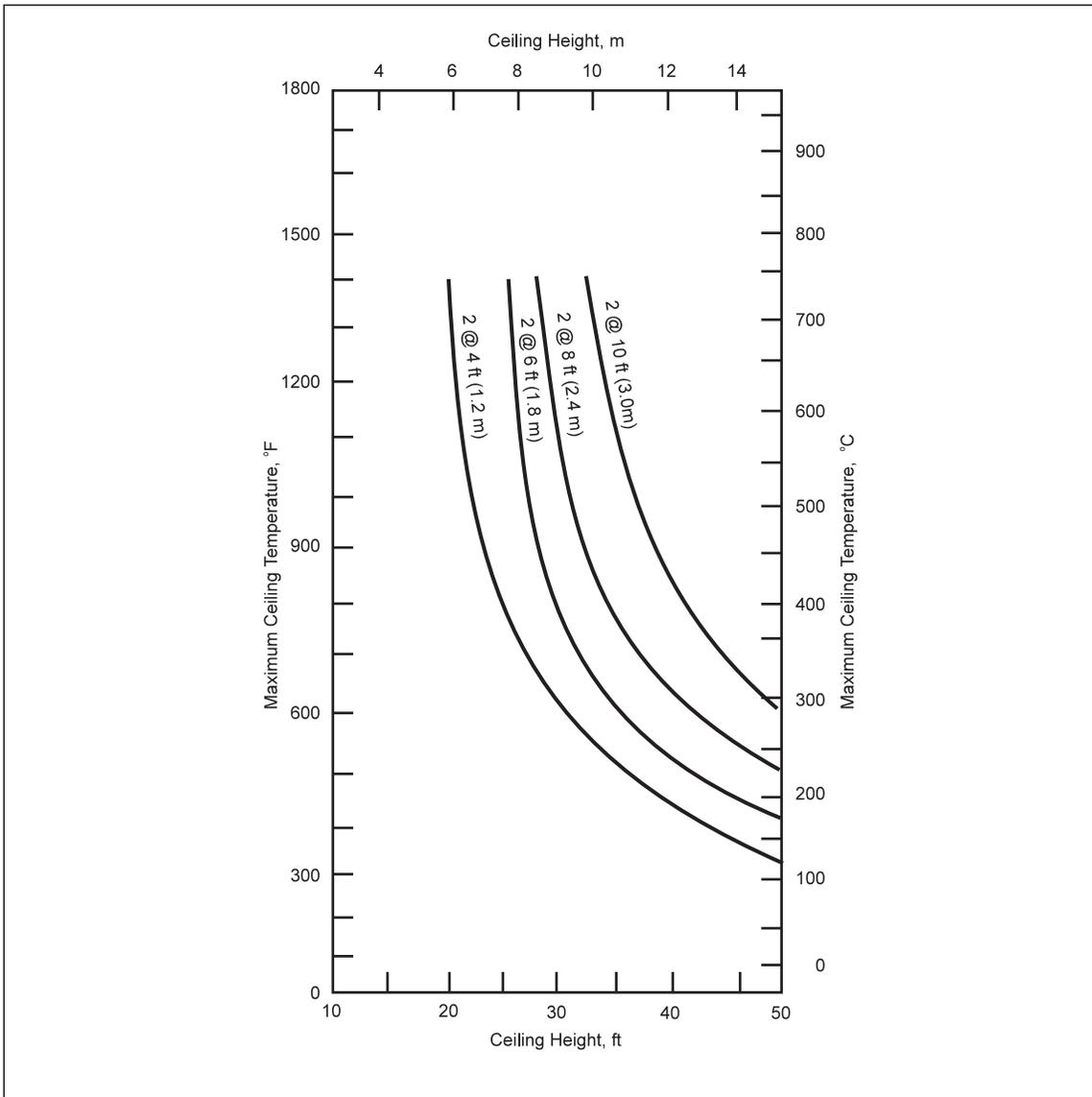
Fig. 3. Ceiling temperatures, double stacks of wood pallets.
