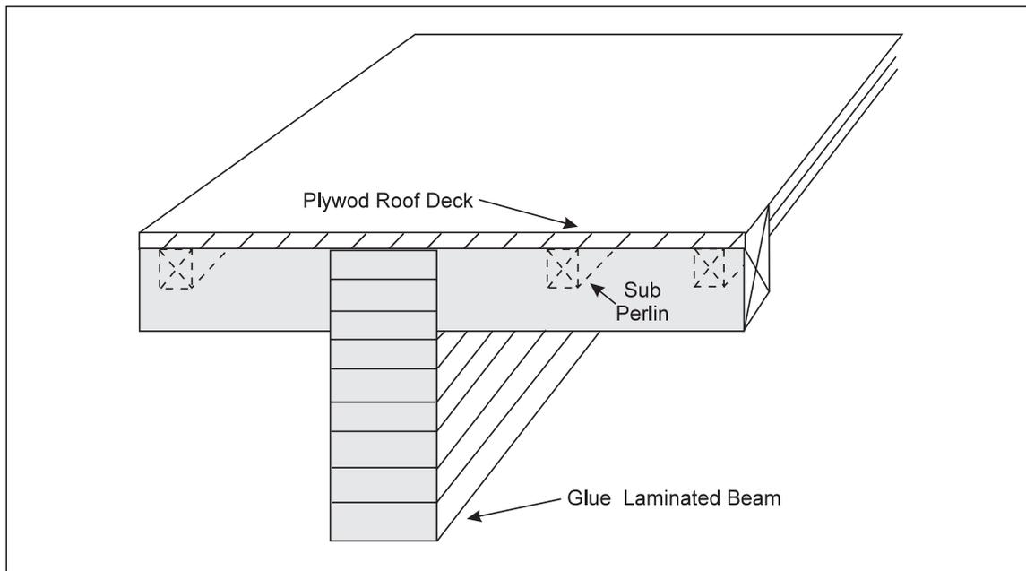
Fig. 15. Typical plywood diaphragm roof deck (not to scale).
