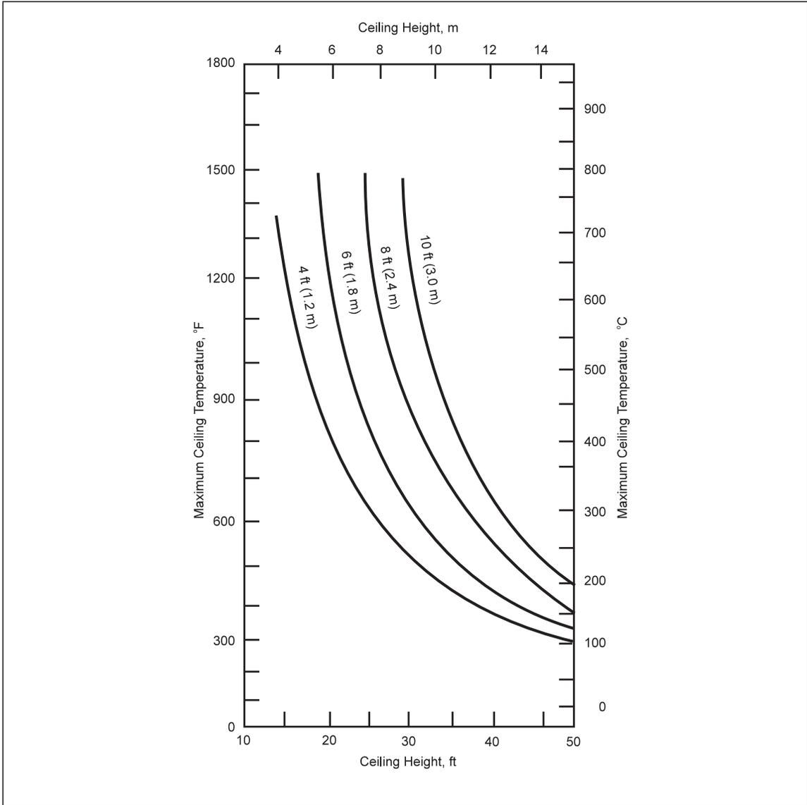
Fig. 4. Ceiling temperatures, single stacks of wood pallets.
