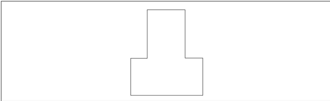
Fig. 8e. Inverted Tee Beam.
