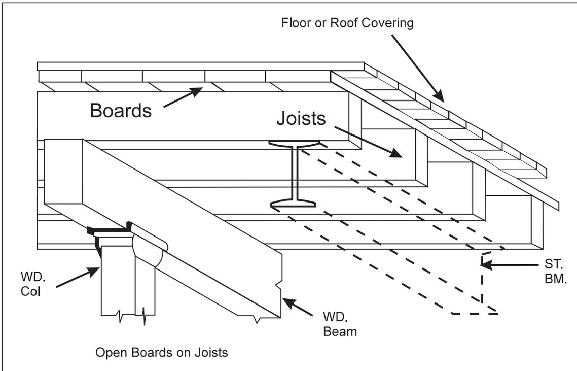
Fig. 13. Open boards on joists.
