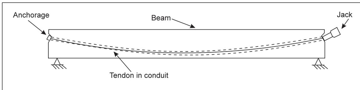
Fig. 9. Post-tensioned concrete beam.
