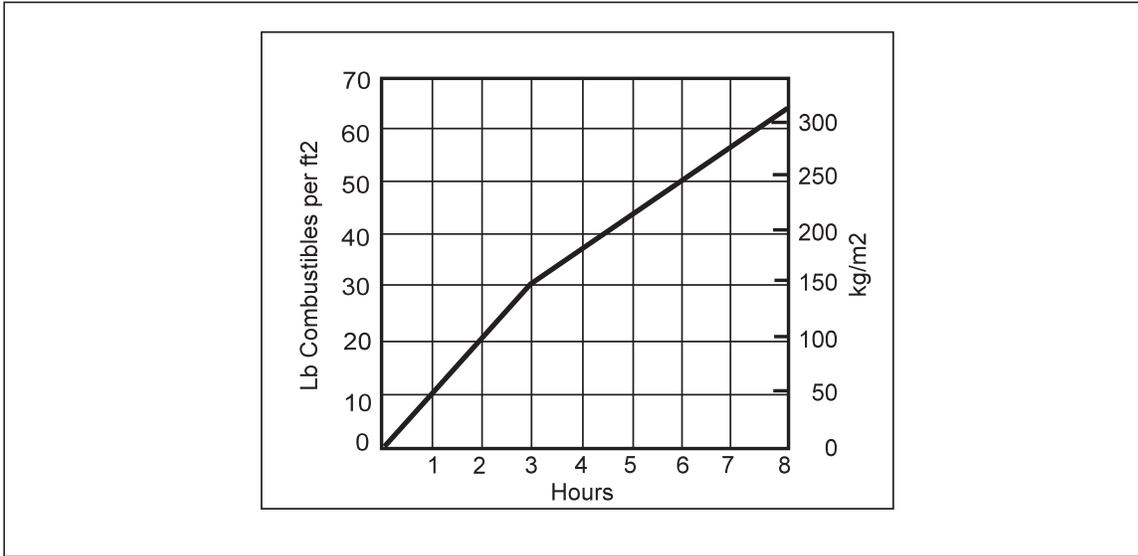
Fig. 1. Weights per square foot and square meters of ordinary (Class A) combustibles required to produce fire severities approximately the ASTM curve for various periods of duration. (Data from Bureau of Standards tests as reported in BM S92.)
