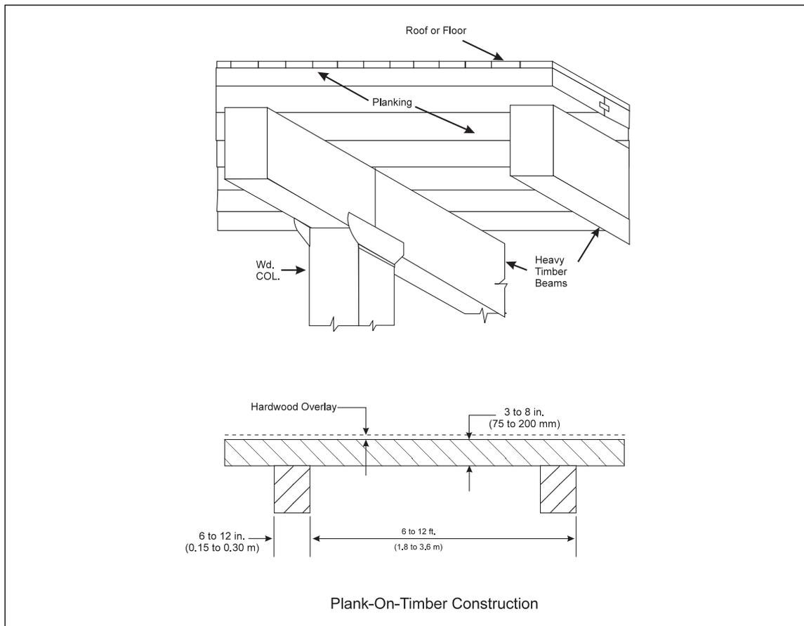
Fig. 12. Plank-on-timber construction.
