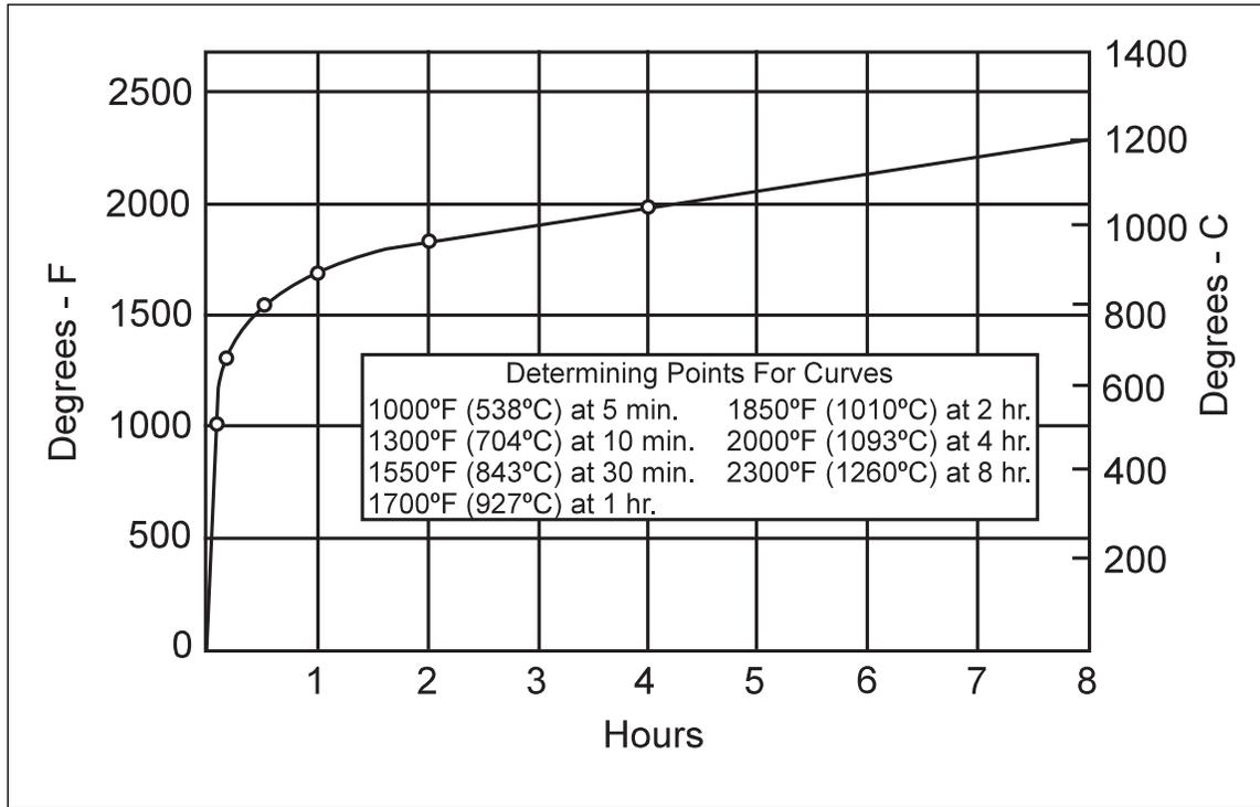
Fig. 4. ASTM E 119 standard time-temperature curve
