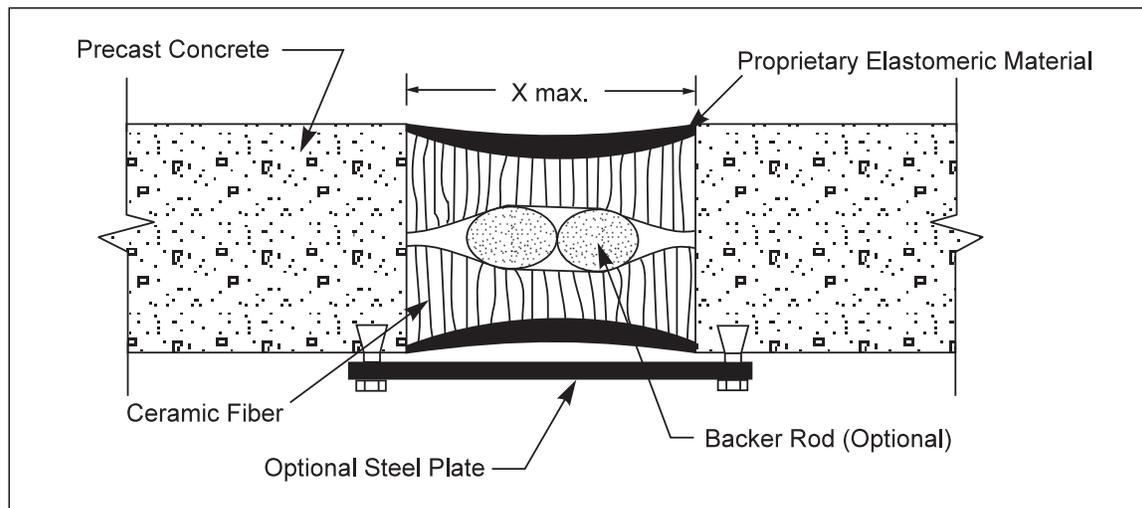
Fig. 3. Section view of proprietary fire-rated joint detail.
