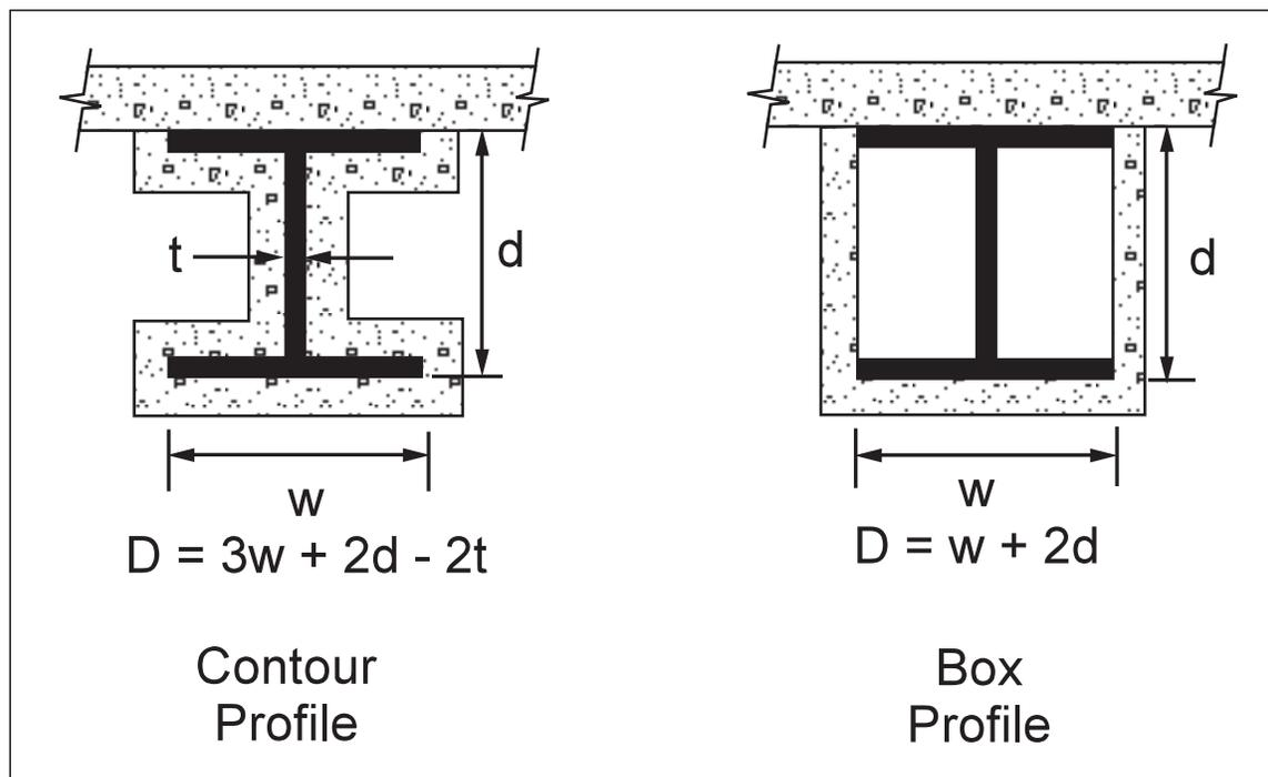
Fig. 1. Heated perimeters for beams
