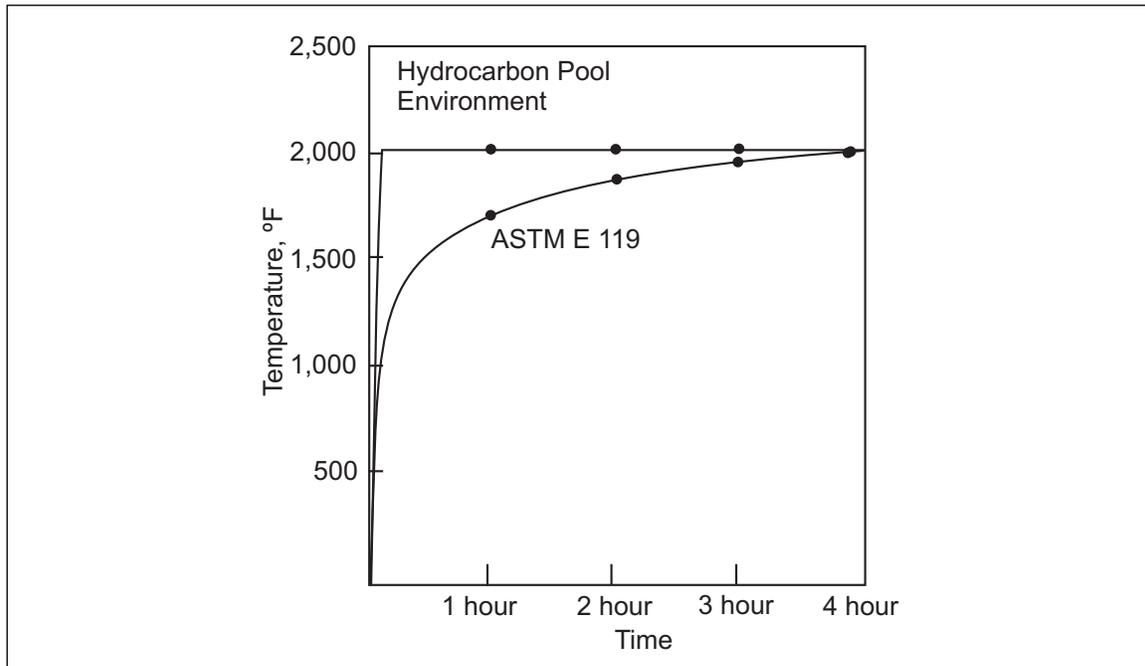
Fig. 5. Comparison of ASTM E 119 time-temperature curve with a hydrocarbon pool fire time-temperature curve
