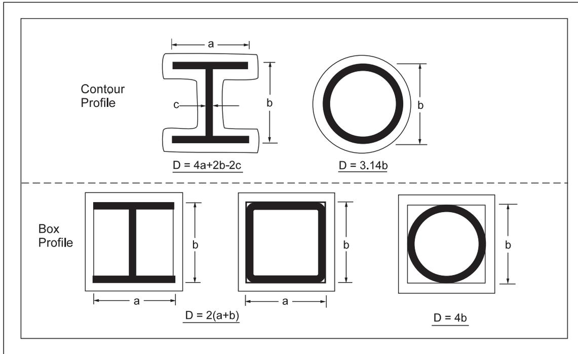
Fig. 2. Column profiles and heated perimeters, D.
