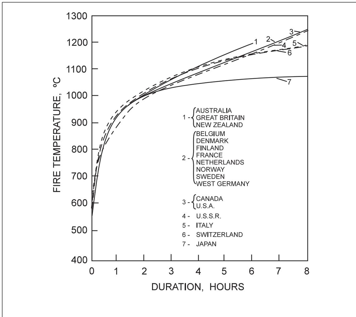
Fig. 6. Time-temperature curves used in various countries
