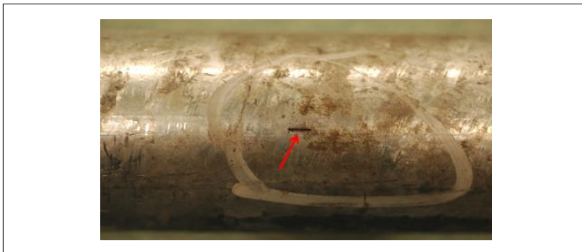
Fig. 14. Preferential grooving corrosion attack surrounding the weld seam area for a preaction system, near the pipe's 6 o'clock (bottom) installed position
