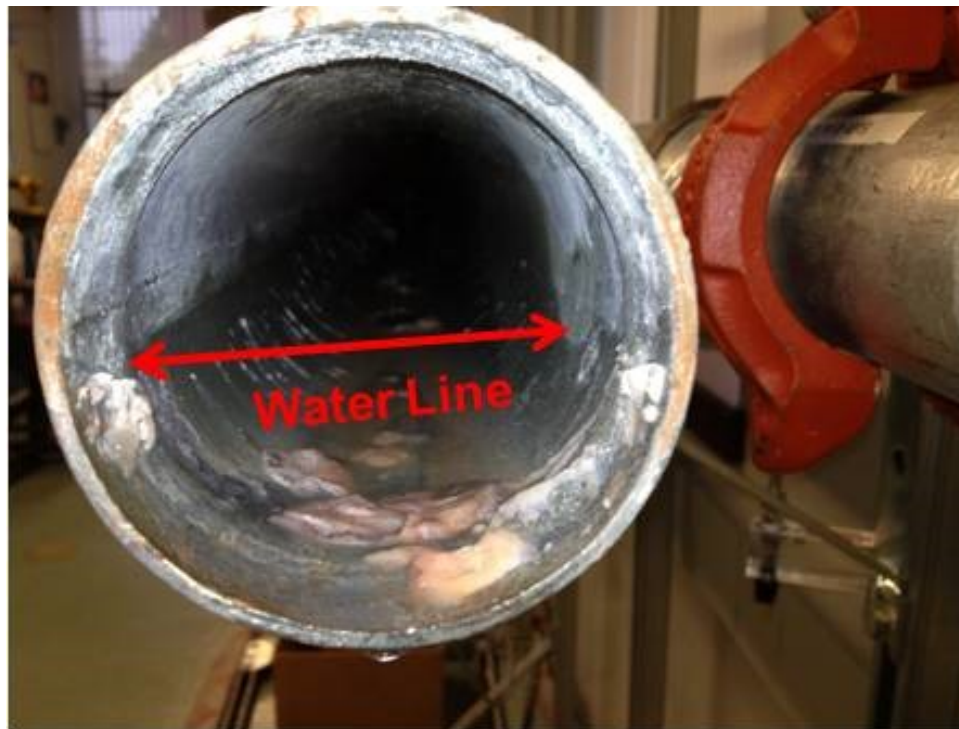
Fig. 4b. Galvanized steel pipe half-filled with compressed nitrogen after nearly six weeks' exposure
