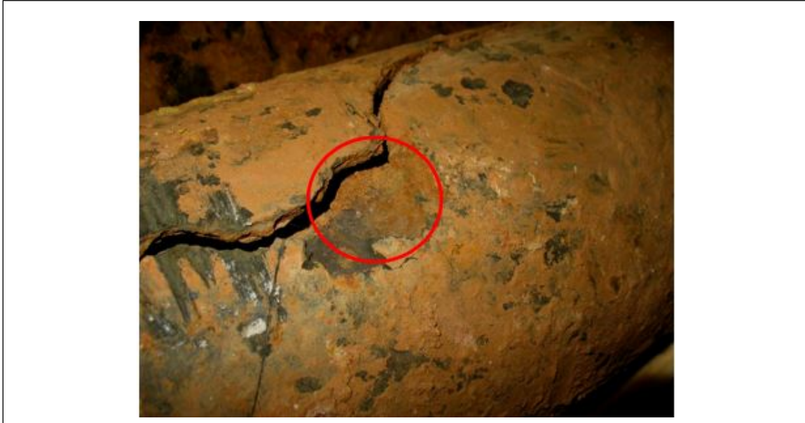
Fig. 7. Ruptured underground water main (identified as gray cast iron, 8 in. [20.3 cm] diameter) with cement lining on its inside diameter
