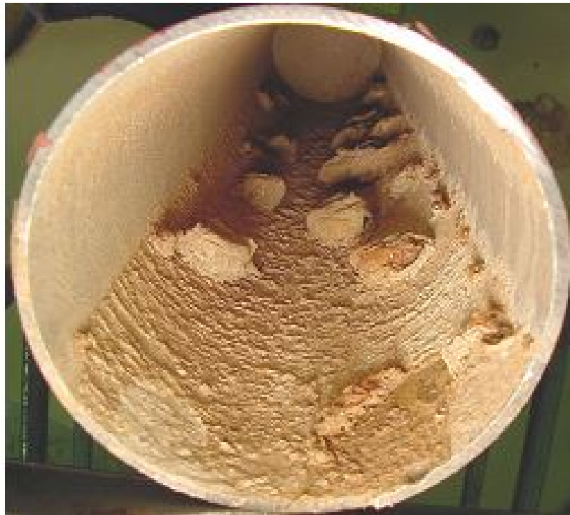
Fig. 9a. Tubercles that formed inside a galvanized steel sprinkler pipe (4 in. [10 cm] diameter)
