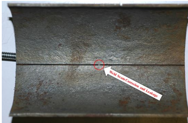
Fig. 12. Preferential grooving corrosion on a pipe weld seam with a .04 in. (1 mm) pinhole leak in a wet pipe system, after removing corrosion products inside an NPS 3 pipe
