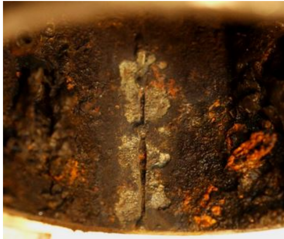
Fig. 11b. Leakage on an NPS 2½ steel sprinkler pipe in a wet pipe system after removal of corrosion products; preferential attack surrounding the weld seam is severe
