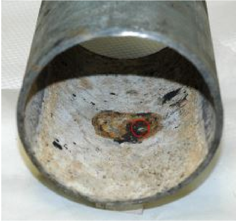
Fig. 9b. Corrosion at the base of a tubercle, which ultimately led to through-wall leakage
