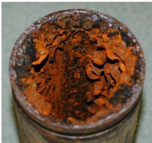
Fig. 15. Corroded steel pipe with many tubercles inside
