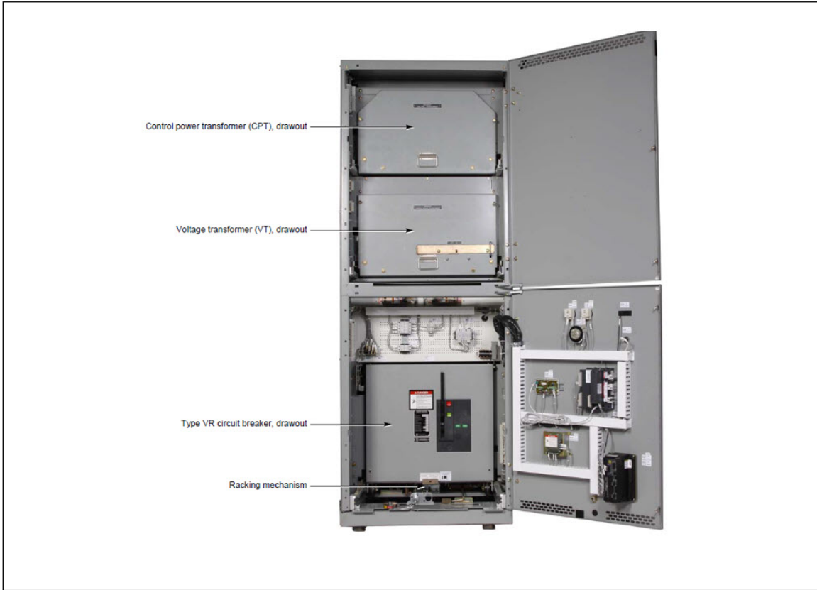
Fig. 2. Front view of typical indoor metal-clad switchgear "Images of Typical Masterclad Metal-Clad Switchgear Assembly and Masterclad Two Bay Assembly—Rear View used with permission from SchneiderElectric. © Schneider Electric. All Rights Reserved. www.schneider-electric.com ".
