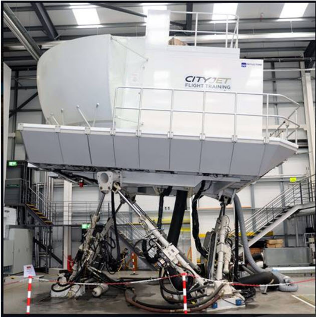
Fig. 3.2-3. View of hydraulic system under simulator module (courtesy of SimTech Aviation)
