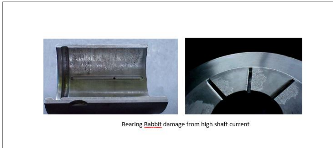
Fig. 4. Examples of damage caused by high level of shaft current (photos courtesy of J. E. Timperley)
