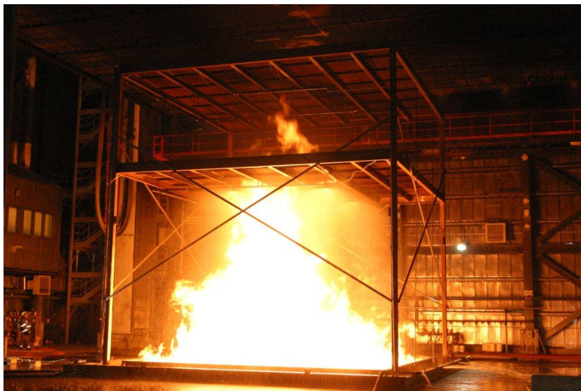
Fig. 15. Process structure test, ethanol fire in 25 ft x 25 ft (7.6 m x 7.6 m) pan with one level of sprinklers
