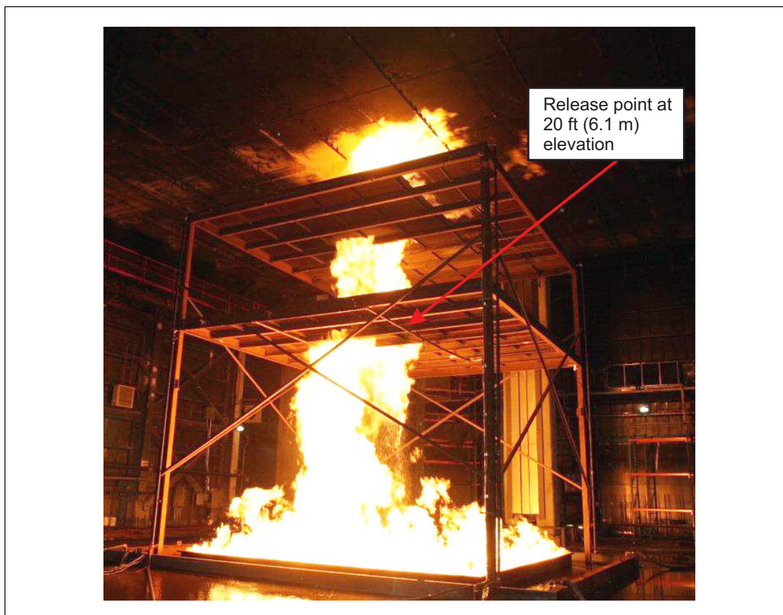
Fig. 17. Three-dimensional spill fire before sprinkler activation (22 gpm [83 L/min] ethanol flow rate)
