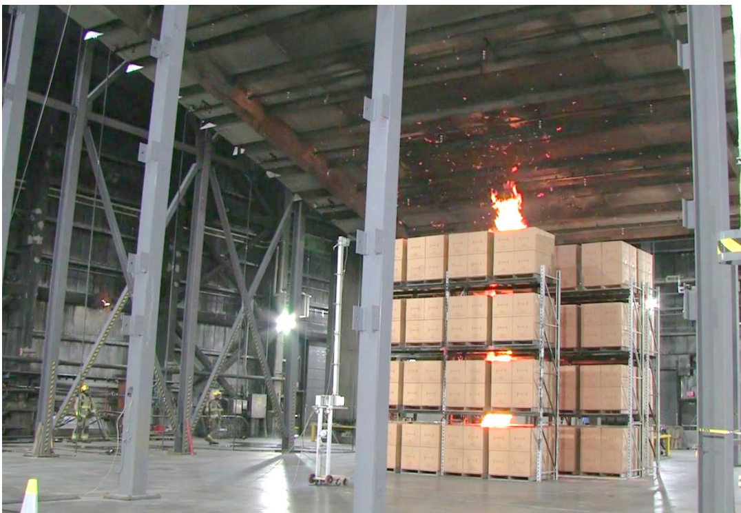
Figure E-36: Test #7 array at 1 min after ignition.
