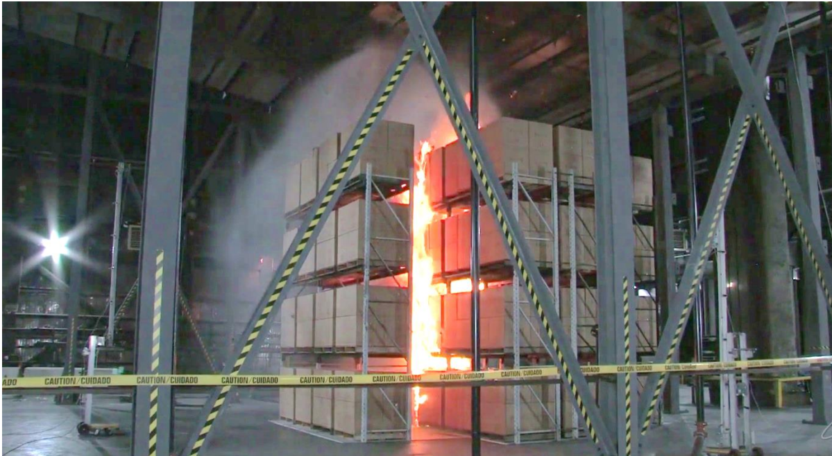
Figure E-19: Test #3 array at 1 min 30 s after ignition.
