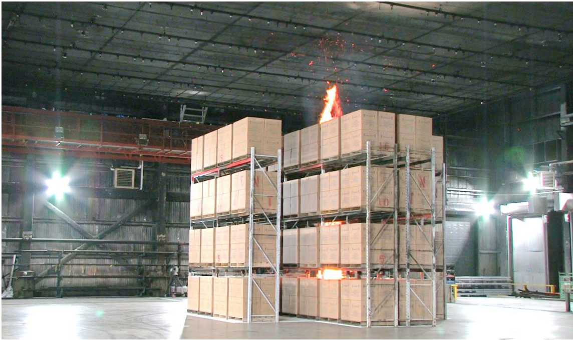
Figure E-1: Baseline test array at 1 min after ignition.
