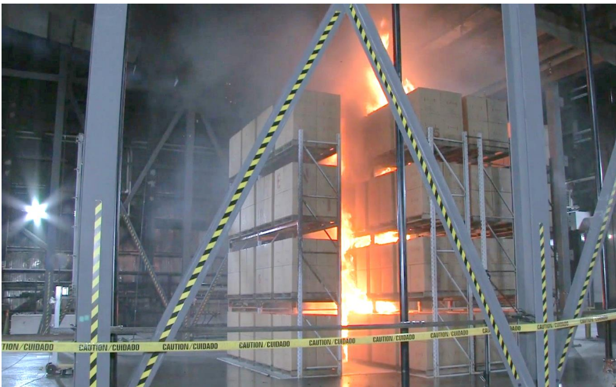
Figure E-30: Test #5 array at 1 min 45 s after ignition.
