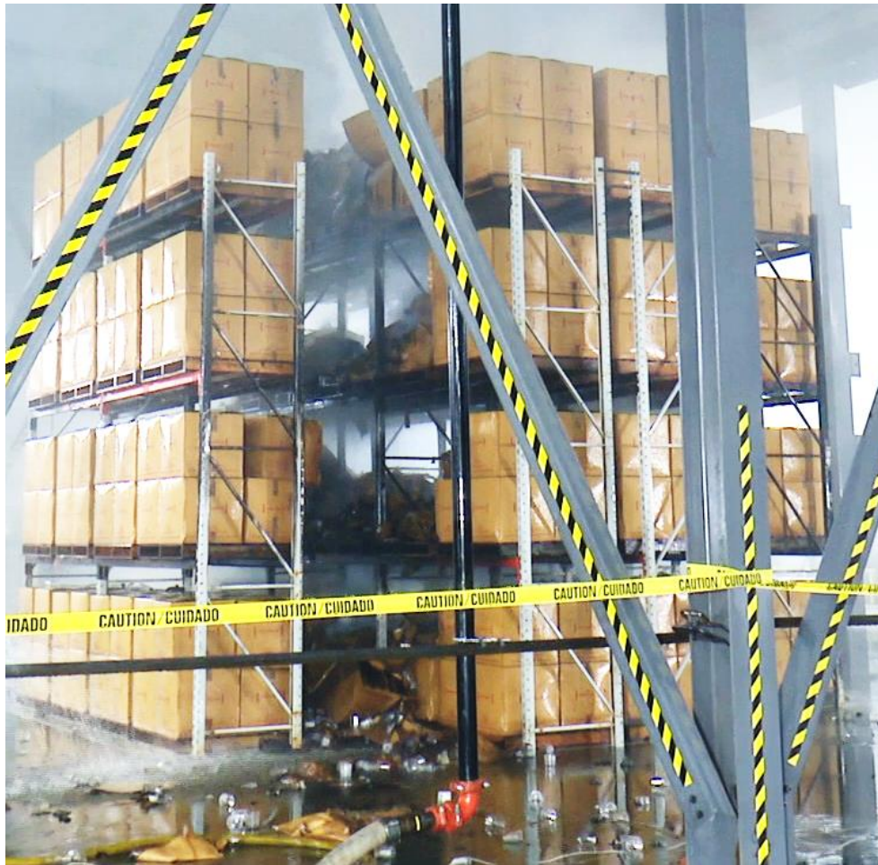
Figure E-16: Test #2 post-test photograph of the east face of the main array showing fire damage.
