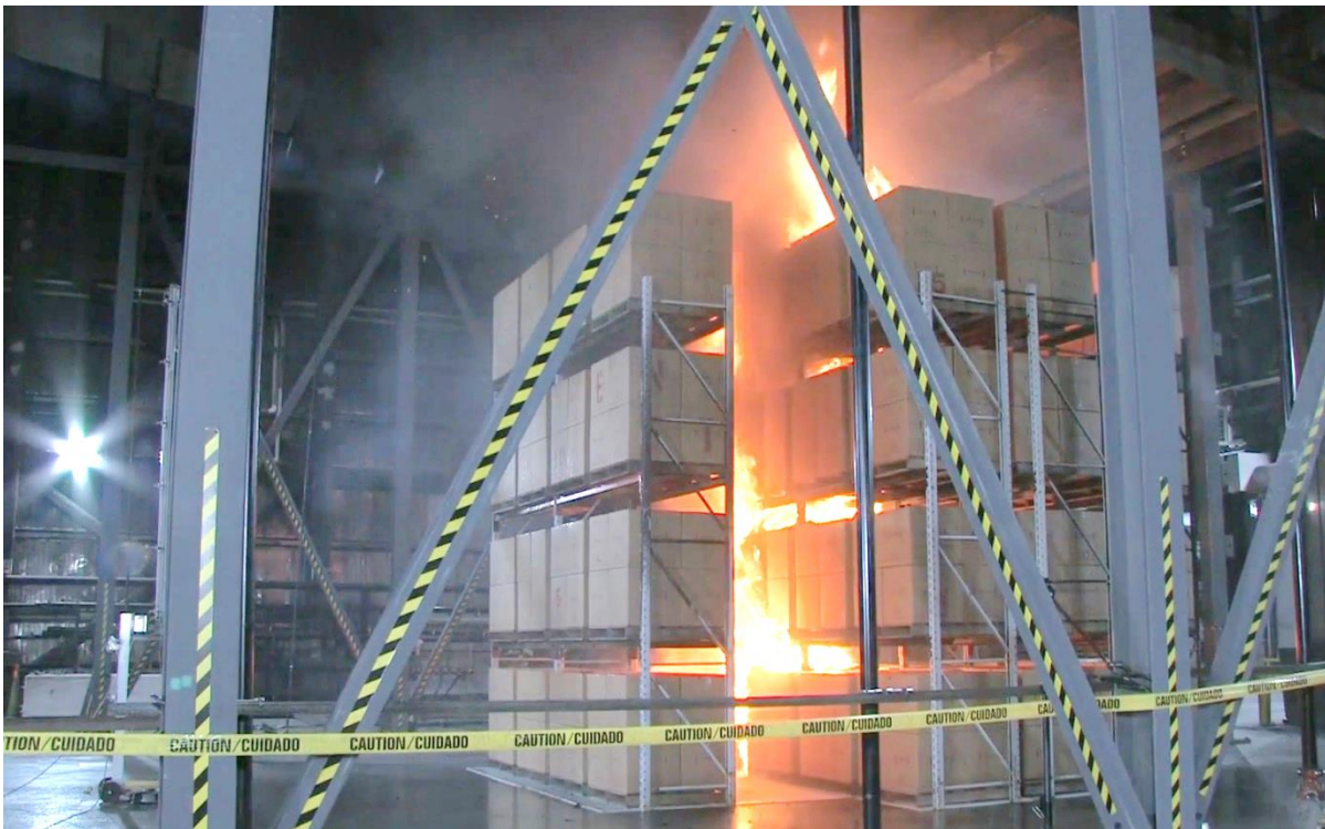
Figure 2-23: Fire on the east side of the main array visible for Test #5 after 1 min 45 s with one sprinkler operating.
