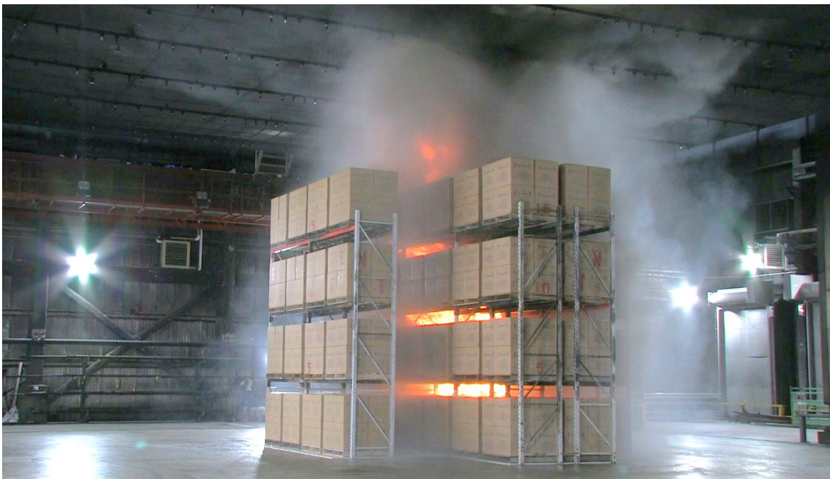
Figure E-3: Baseline test array at 1 min 30 s after ignition.
