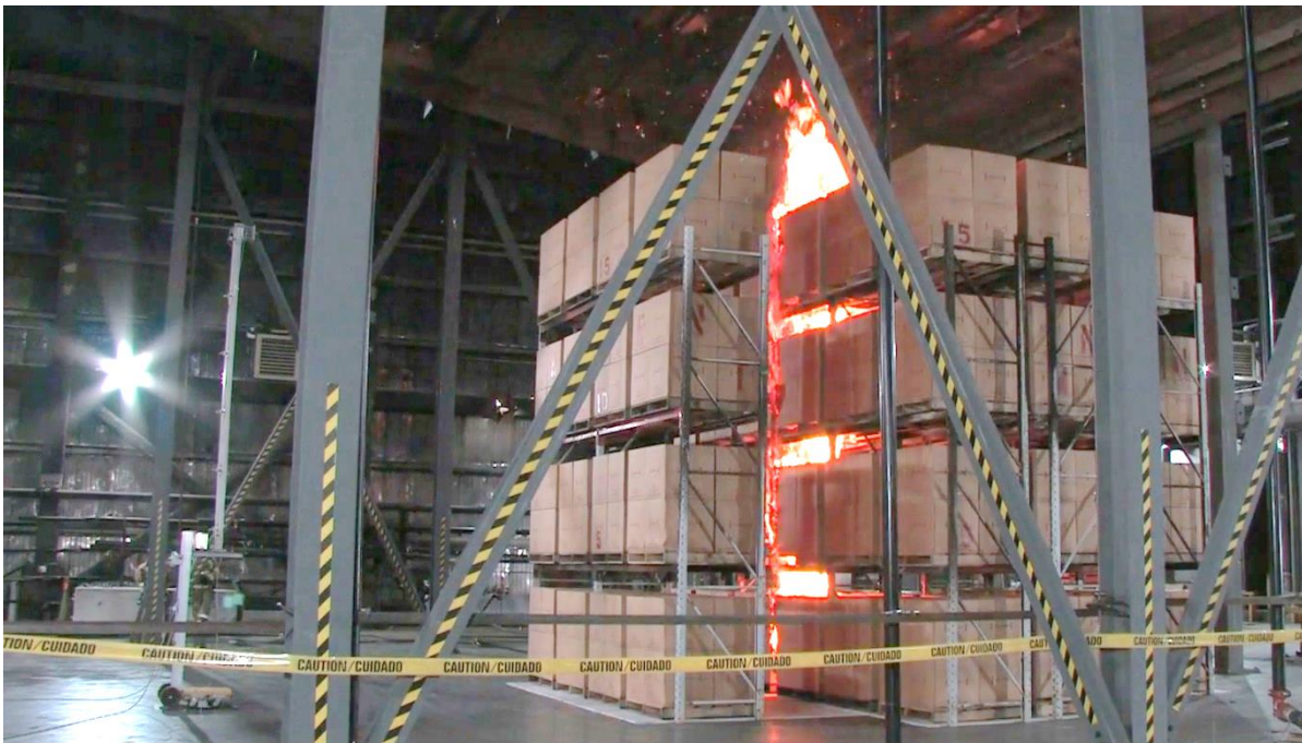
Figure E-32: Test #6 array at 1 min after ignition.
