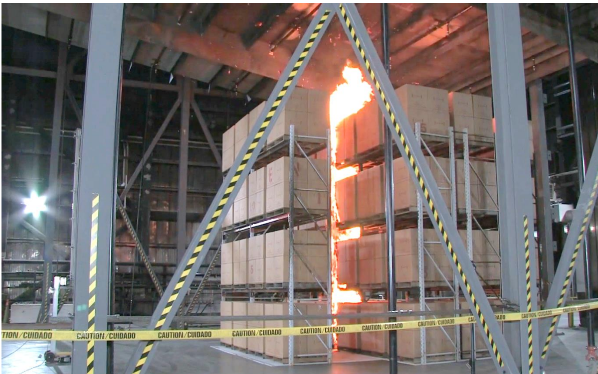
Figure E-28: Test #5 array at 1 min 15 s after ignition.
