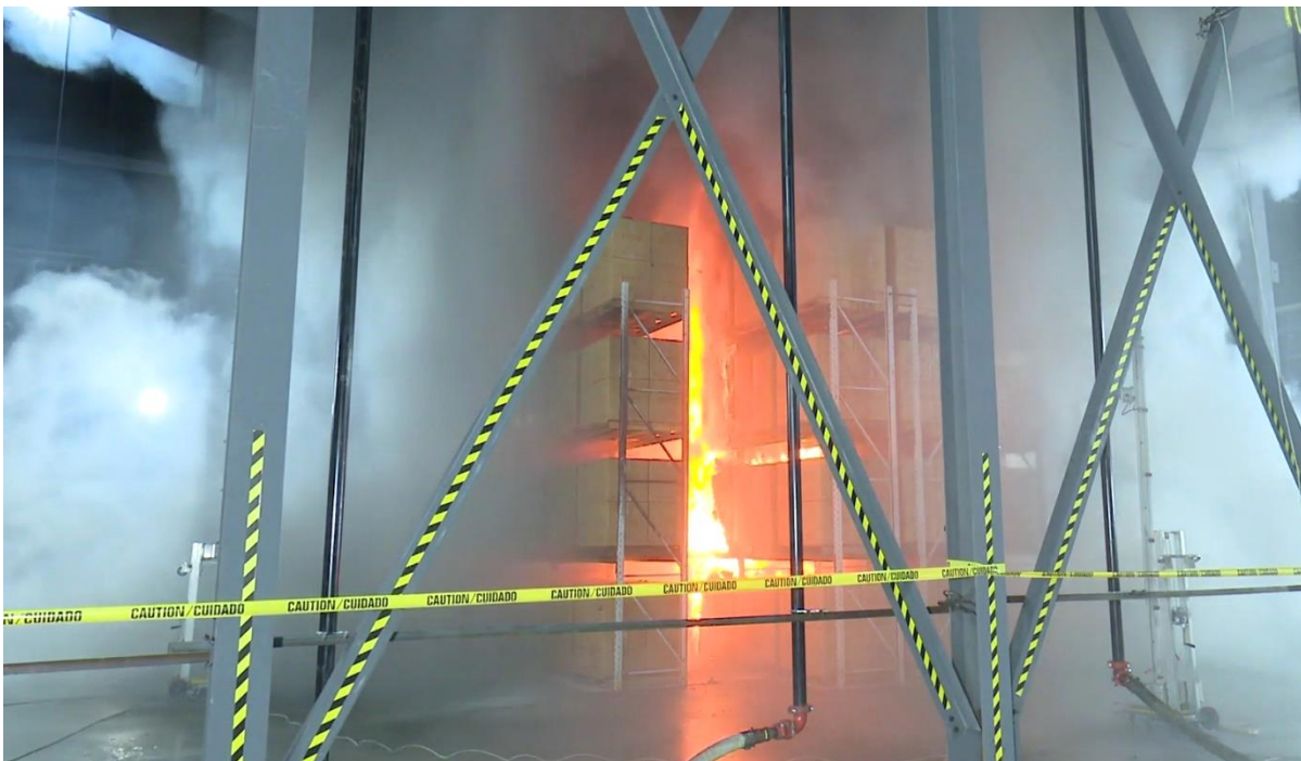
Figure E-15: Test #2 array at 1 min 45 s after ignition.
