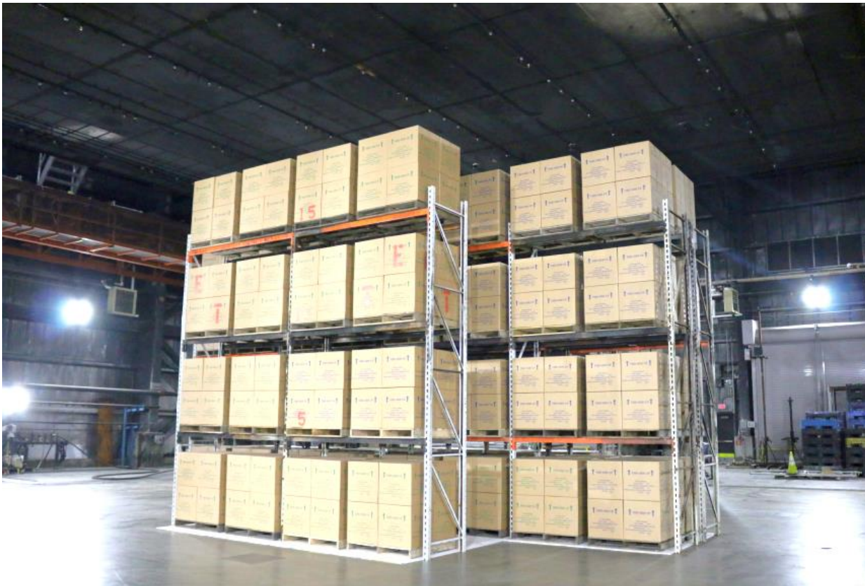
Figure 2-5: Photograph of the CUP arrays for the baseline test.
