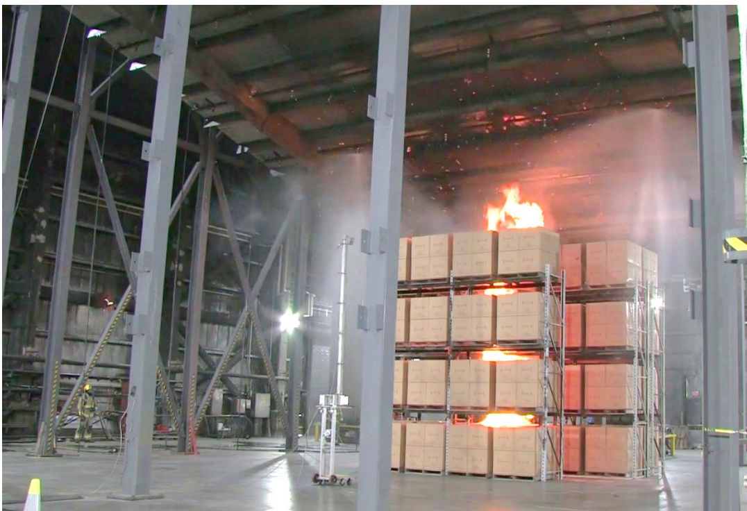
Figure E-37: Test #7 array at 1 min 15 s after ignition.
