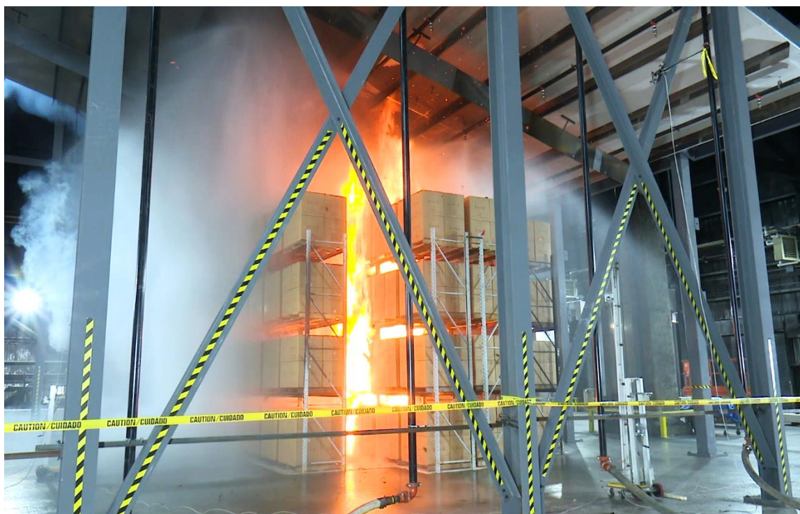
Figure 2-36: Test #2 fire on the east face and above the main array 1 min 30 s after ignition
