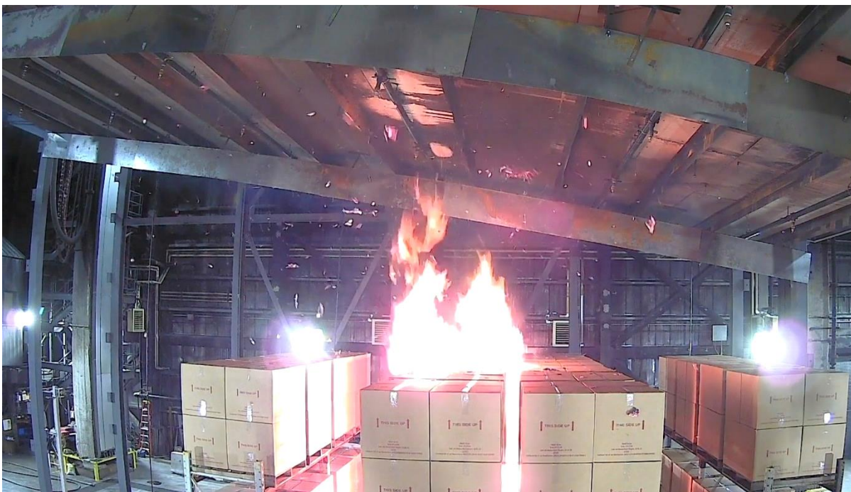
Figure E-23: Test #4 array at 1 min 15 s after ignition.
