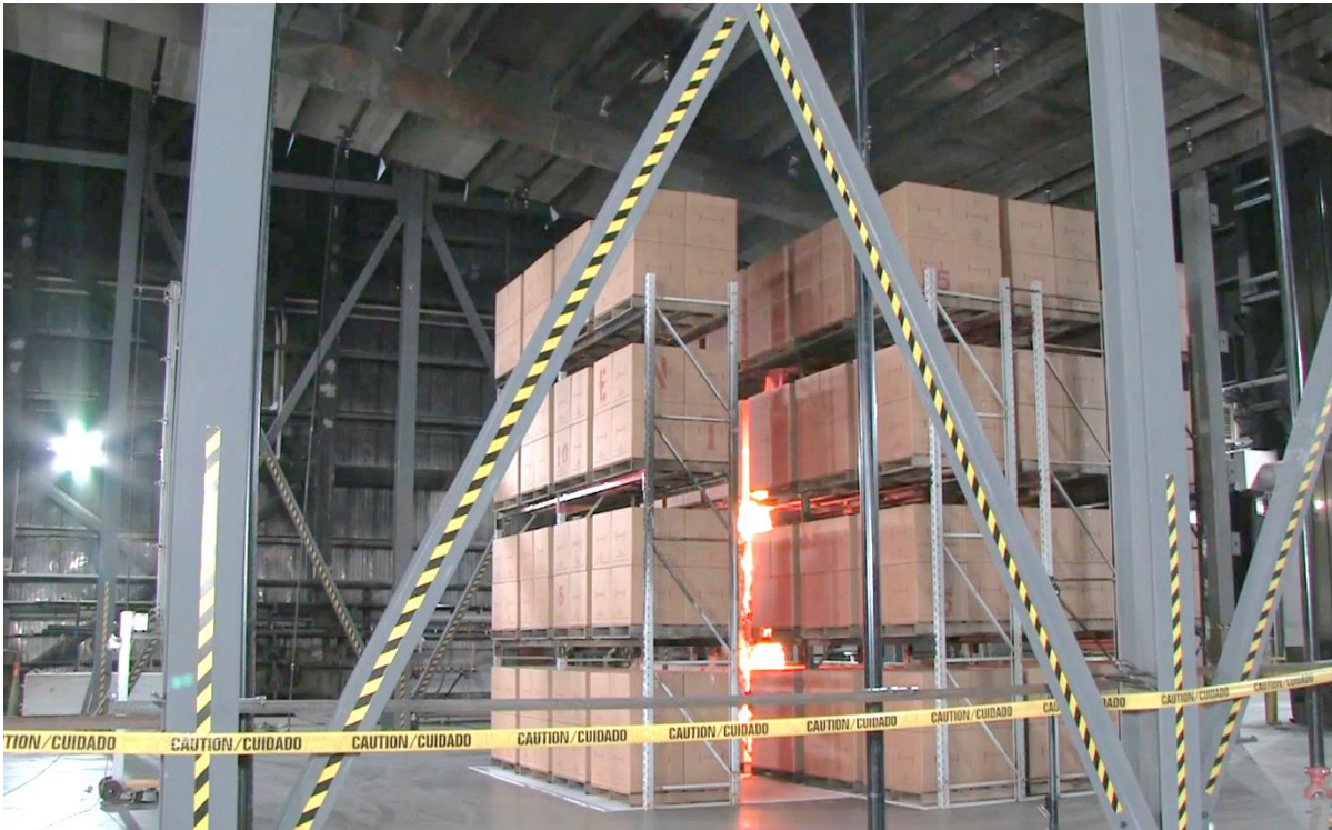
Figure E-27: Test #5 array at 1 min after ignition.
