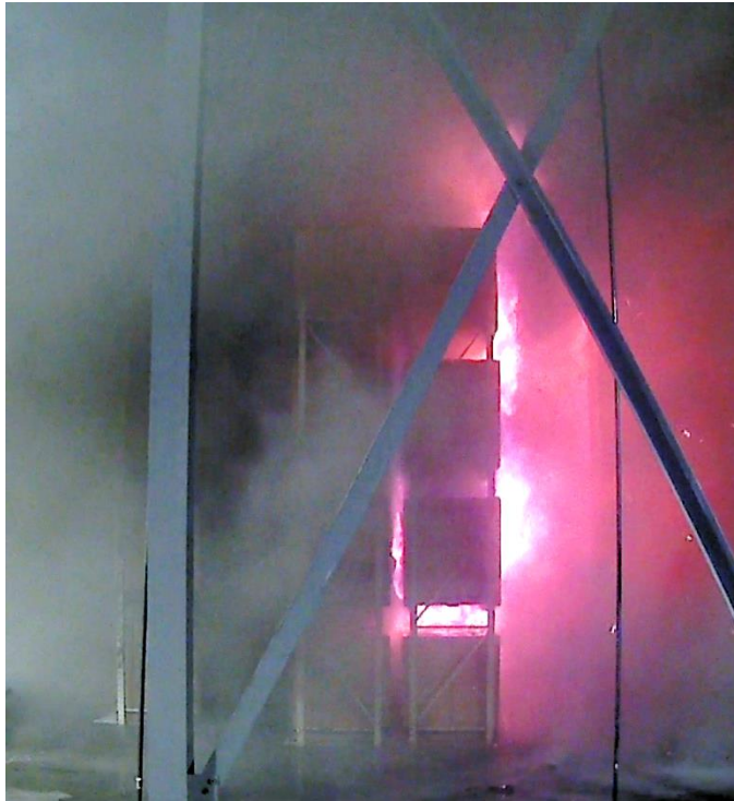
Figure 2-24: Test #5 side view of the south end of the main array 4 min after ignition. Intense burning of the commodity can be observed. Spray from the closest sprinkler is obstructed by the adjacent girder.
