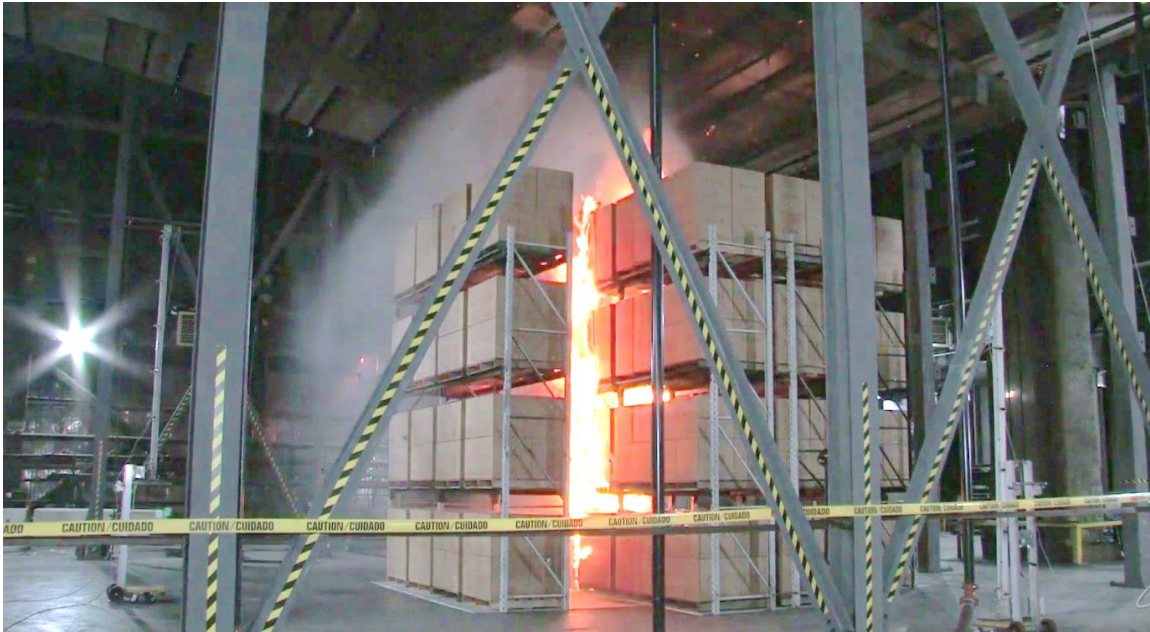
Figure 2-12: Test #3 fire on east face of main array at 1 min 30 s after ignition.
