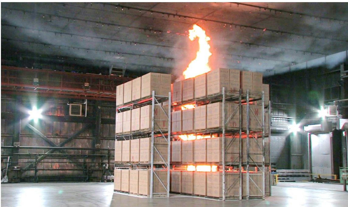
Figure E-2: Baseline test array at 1 min 20 s after ignition.
