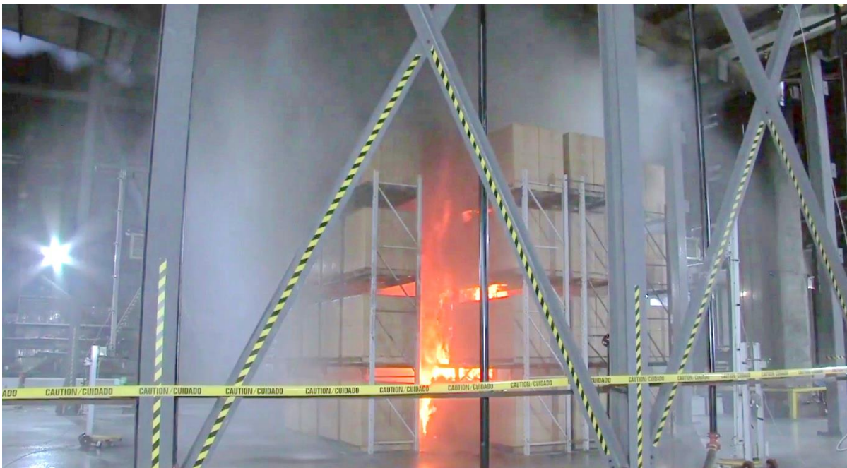
Figure E-20: Test #3 array at 1 min 45 s after ignition.
