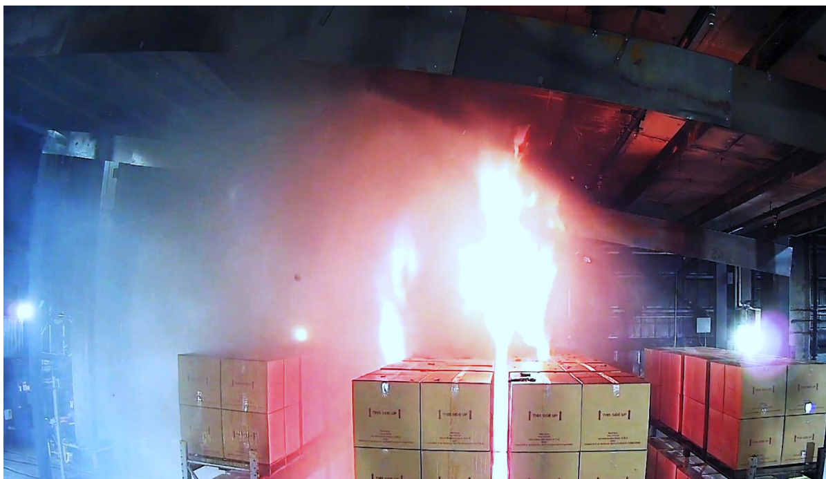
Figure 2-17: Test #4 – fire above the main array at 1 min 30 s after ignition. Two sprinklers in the upslope direction were operating.
