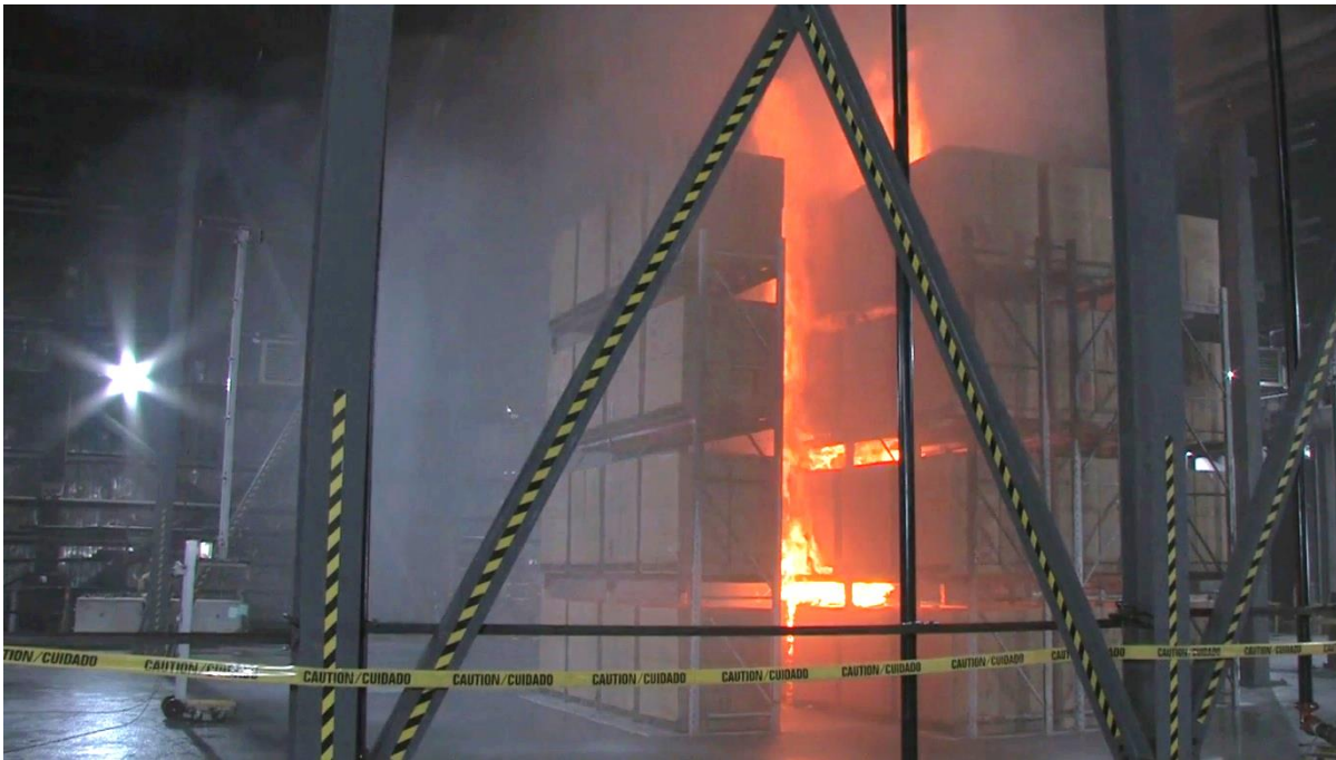
Figure E-34: Test #6 array at 1 min 30 s after ignition.
