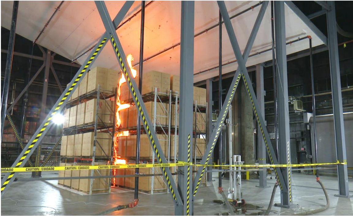
(a) Fire visible on the east face and above the main array 1 min after ignition
