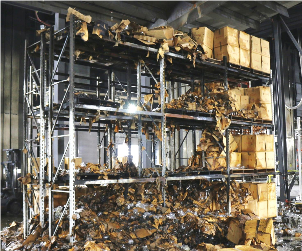
Figure E-31: Test #5 post-test photograph of the east face of the main array showing fire damage.
