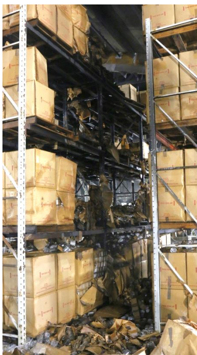
Figure E-39: Test #7 post-test close-up photograph of the east face of the main array showing fire damage.
