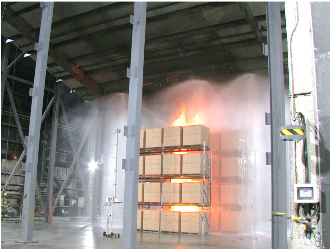
Figure 2-40: Test #7 fire on the east face and above the main array 1 min 20 s after ignition
