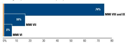
As illustrated here, the Northridge earthquake demonstrated that sprinkler systems can fail at earthquake intensity levels above MMI VI when not braced as recommended by FM Global.
