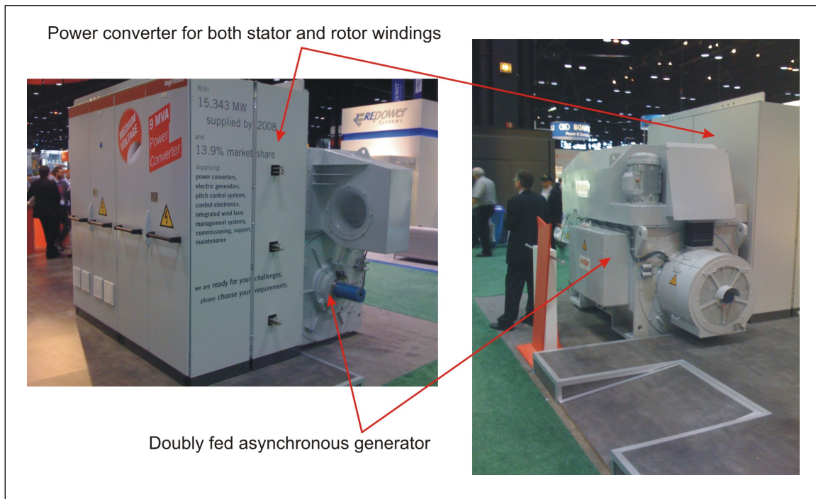
Fig. 3.4.3-2. A 1.5MW doubly fed asynchronous generator connected to an air cooled, IGBT with PWM power converter
