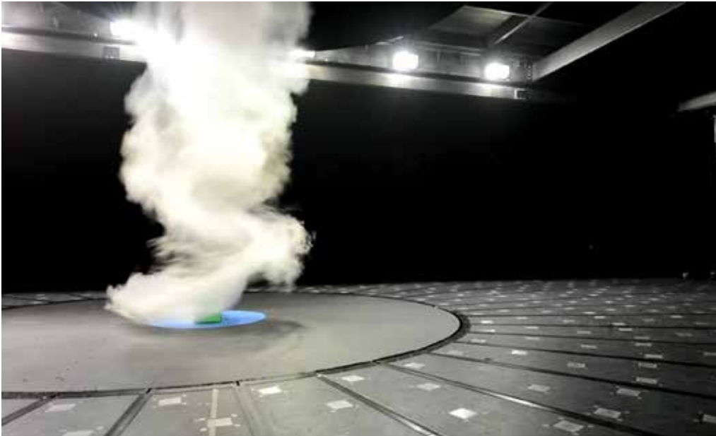
FIGURE 5: A lab tornado interacting with a model building. Picture provided by the WindEEE Research Institute at Western University.
